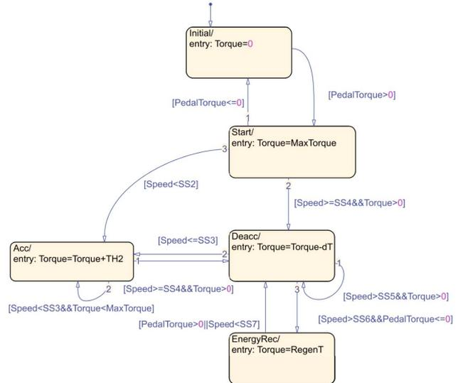
Figure 3. ECU control algorithm
