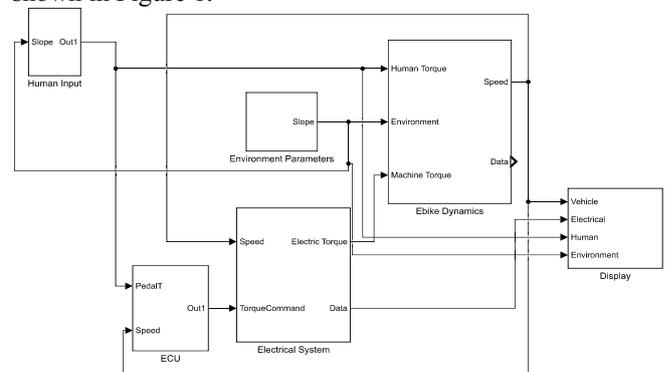
Figure 1. Block diagram of the modeled ebike
