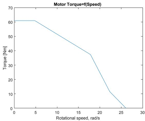
Figure 4. Used motor torque/speed diagram
