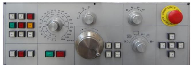
Fig. 2. Control panel of the turning machine.
