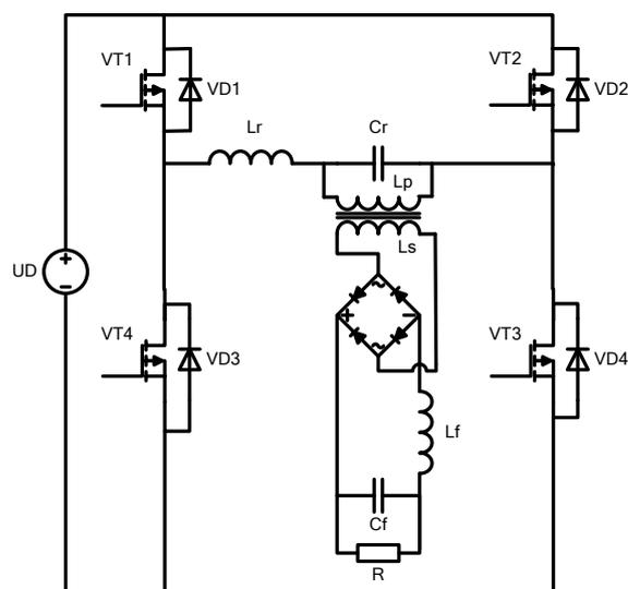
Fig. 4. Series resonant parallel-loaded DC-DC converter.
