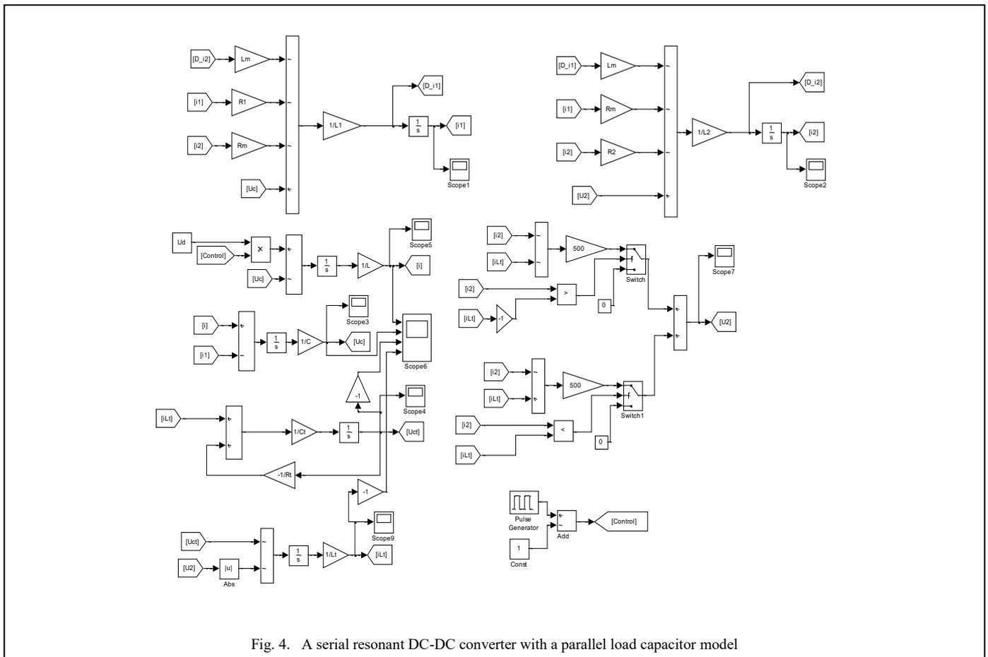
Fig. 4. A serial resonant DC-DC converter with a parallel load capacitor model
