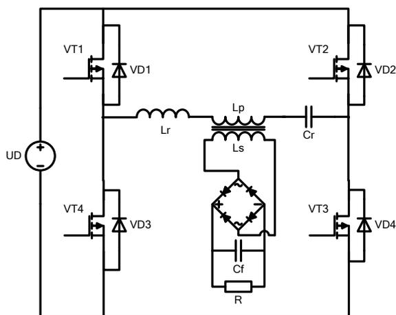
Fig. 3. Series resonant DC-DC converter.
