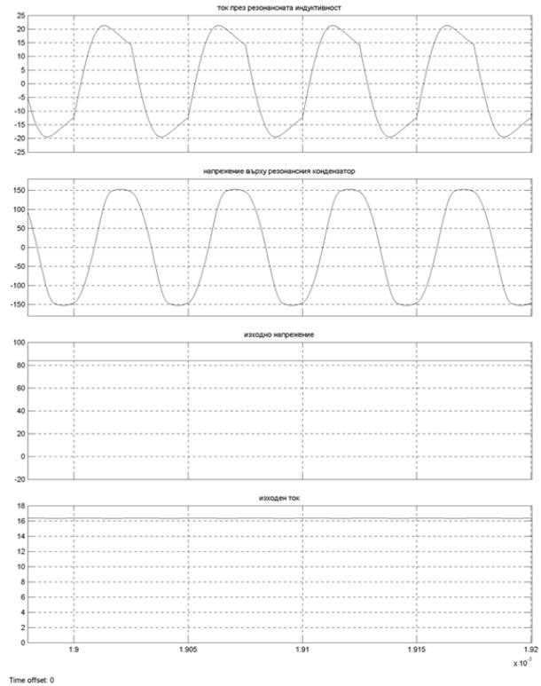
Fig. 6. Results from the simulation of the serial resonant DC-DC converter with parallel loaded capacitor
