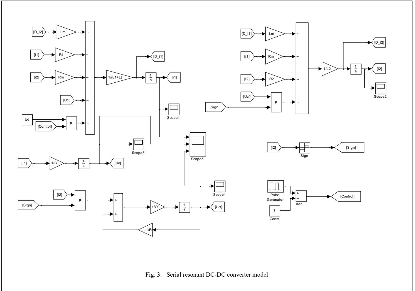
Fig. 3. Serial resonant DC-DC converter model
