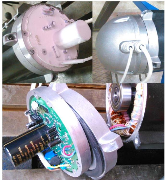
Fig. 7 Electronics integrated inside the motor
