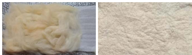
Fig. 9. Fiber laying method and finished look of Sample 3
