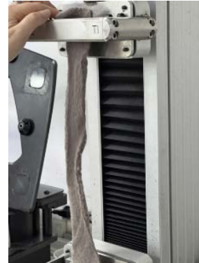
Fig. 13. Test to determine the strength and elongation
