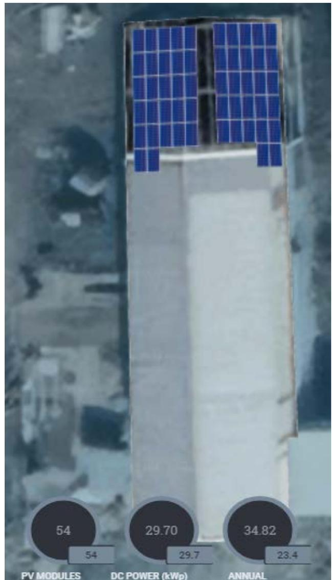
Fig. 4. Placement of panels at power 30 kWp.
