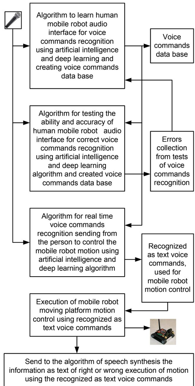
Fig. 2. The proposed voice commands recognition algorithm in human mobile robot audio communication interface developed with usage of AI and neural networks with DL
