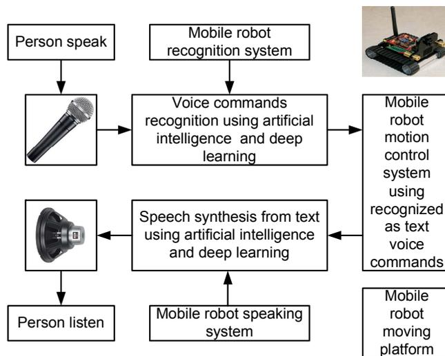
Fig. 1. Block schema of the proposed human mobile robot audio communication interface developed with usage of AI and neural networks with DL
