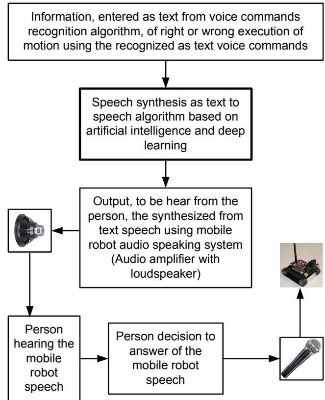
Fig. 3. The proposed speech synthesis algorithm in human mobile robot audio communication interface developed with usage of AI and neural networks with DL
