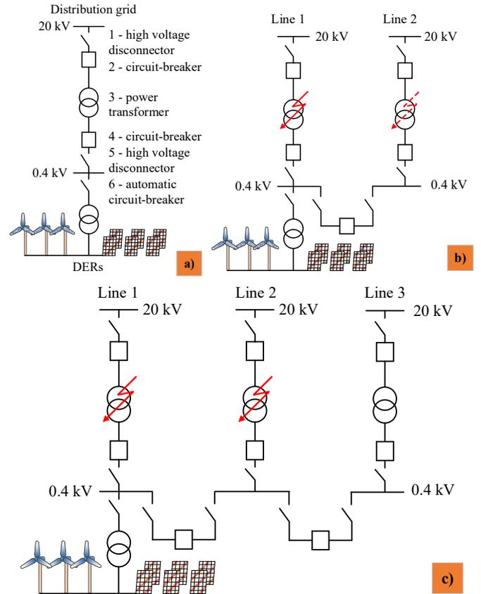
Fig. 3. Decentralized energy system with two substations
