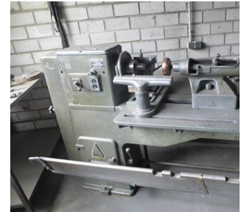
Fig.3b Layfield DB 20 Spinning Lathe 1956, 225-2800rpm [9]
