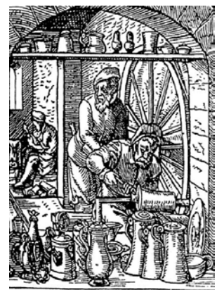
Fig. 2 Wooden spinning lathe with a manually operated flywheel to spin the workpiece [3]
