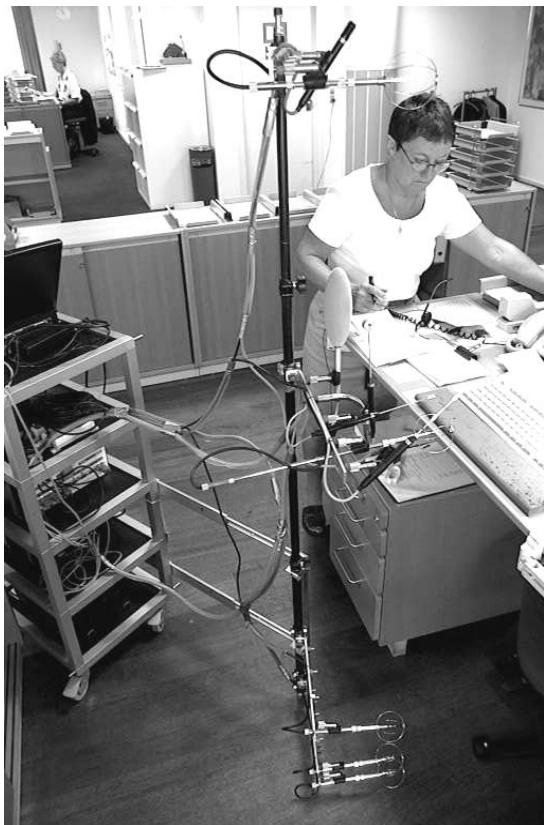
Figure 1. Mobile measurement unit
