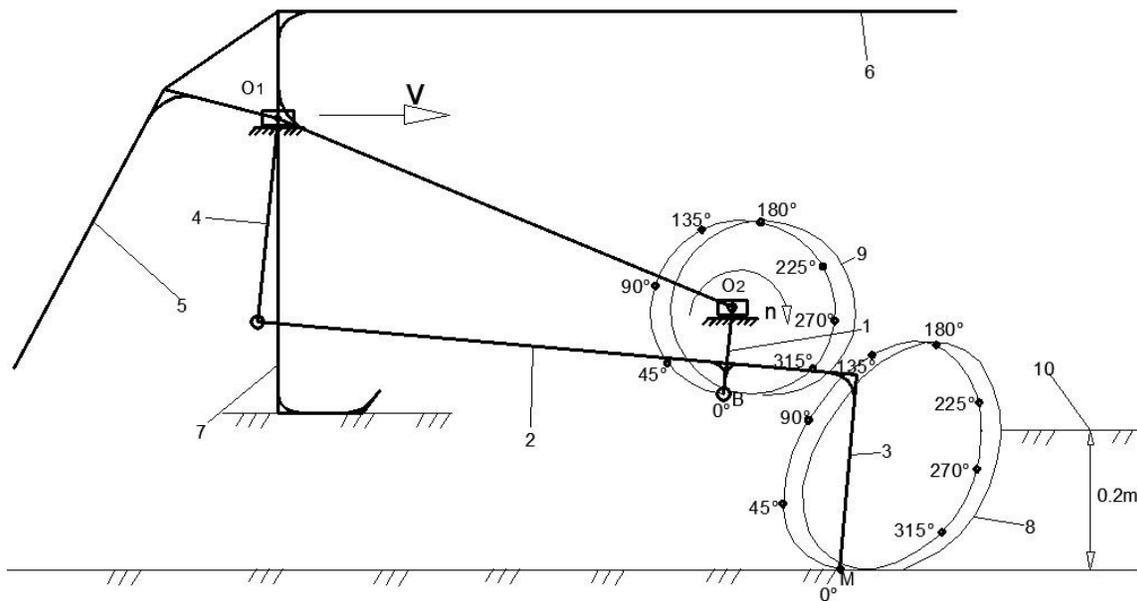
**FIGURE 2.** Diagram of a spading machine with horizontal arm:
