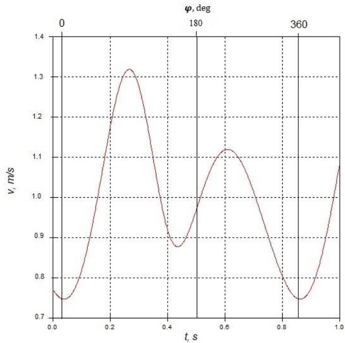
**FIGURE 3.** Diagrams for absolute velocity  $V$  at point  $M$  in the mechanism of the spading machine according to the angle  $\varphi$  of rotation of the machine crankshaft
