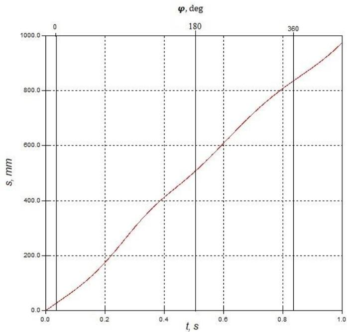
**FIGURE 4.** Diagrams for passed path at point  $M$  in the mechanism of the spading machine according to the angle  $\varphi$  of rotation of the machine crankshaft
