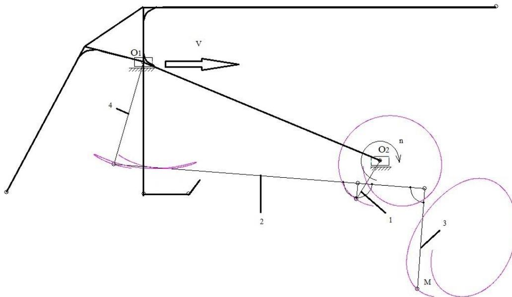
**FIGURE 1.** Using the software product SAM for synthesizing a kinematic model of a spading machine with horizontal arm: 1 – crankshaft; 2 – arm; 3 – working body (shovel); 4 – timing bar.
