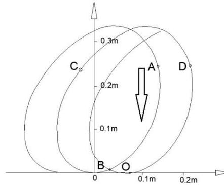
**FIGURE 5.** Trajectory of point M on the working body of the spading machine with horizontal arm.
