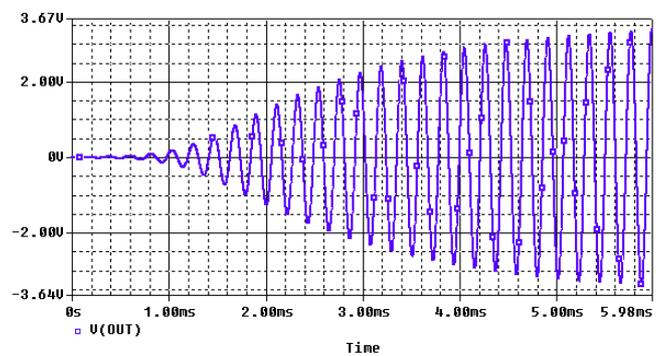
Fig. 10. Diagram of output voltage,  $a_{M3} = a_{M4} = 0,3$  and  $a_{M1} = a_{M2} = 0,05$
