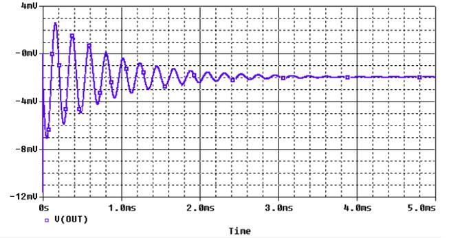
Fig. 3. Time diagram of output voltage of the generator at  $a_{M3} = 0,4$
