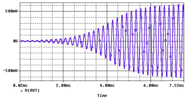
Fig. 4. Time diagram of output voltage of the generator at  $a_{M3} = 0,35$
