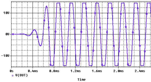
Fig. 6. Time diagram of output voltage of the generator at  $a_{M3} = 0,05$
