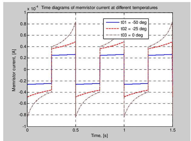
**Fig. 8.** Time diagram of memristor current at temperatures -50, -25 and 0 degrees Celsius
