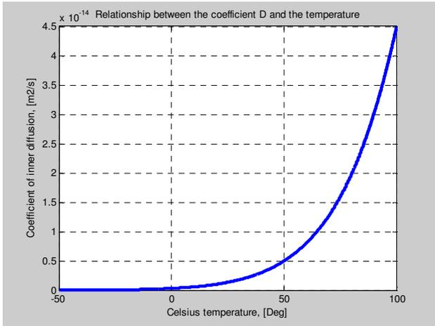
**Fig. 16.** Relationship between the coefficient of inner diffusion  $D$  and the Celsius temperature
