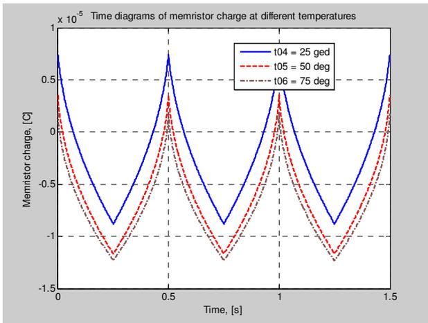
**Fig. 11.** Time diagram of memristor charge  $q$  at temperatures 25, 50 and 75 degrees Celsius, at  $q_{i0}/Q_d = 0,7$
