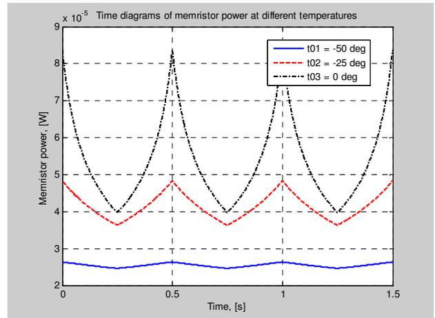
**Fig. 13.** Time diagrams of the memristor power consumed at temperatures -50, -25 and 0 degrees Celsius
