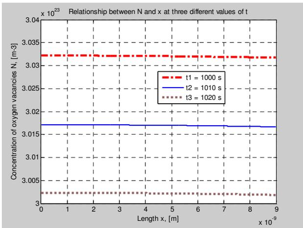
**Fig. 17.** Relationship between the concentration of oxygen vacancies  $N$  and the length of penetration of the charges
