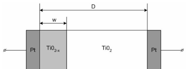
**Fig. 15.** Structure scheme of a titanium-dioxide memristor
