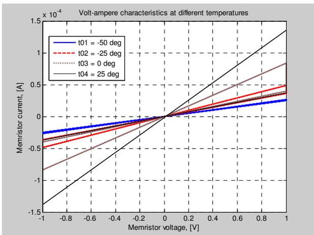
**Fig. 12.** Volt-ampere characteristics of the memristor at several different Celsius temperatures
