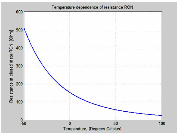
Fig. 3. Dependence between memristors' resistance in closed state  $R_{ON}$  and the Celsius temperature  $t^\circ$
