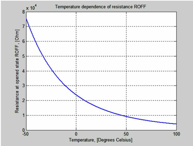
Fig. 2. Dependence between memristors' resistance in opened state  $R_{OFF}$  and the Celsius temperature  $t^\circ$
