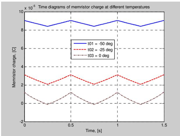
**Fig. 10.** Time diagram of memristor charge  $q$  at temperatures -50, -25 and 0 degrees Celsius, at  $q_{i0}/Q_d = 0,5$
