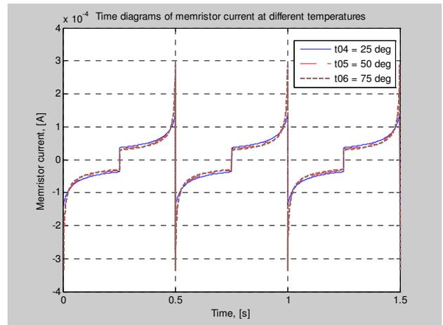
**Fig. 9.** Time diagram of memristor current at temperatures 25, 50 and 75 degrees Celsius
