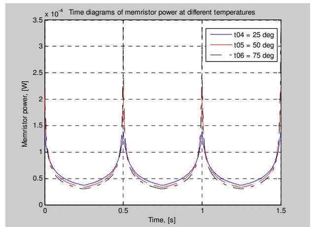
**Fig. 14.** Time diagrams of the memristor power consumed at temperatures 25, 50 and 75 degrees Celsius
