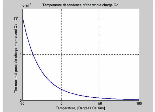
Fig. 4. Dependence between memristors' full possible charge memorized  $Q_d$  and the Celsius temperature  $t^\circ$
