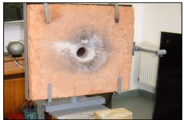
Fig. 7. Experimental system with the possibility of creating a radial jet-front view.
