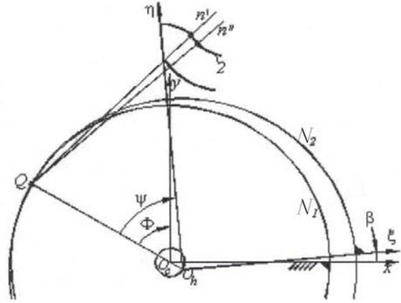
Fig. 3 Generating Two Families of Curves in Plane of Centroids
