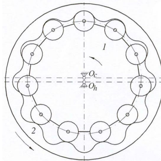
Fig. 1 Compound Pinion with Cylindrical Teeth and Epicycloidal Gear with  $m=3.5$  mm,  $N_1 = 11$ ,  $N_2 = 12$ ,  $x=0.2$  and  $r_c^* = 1$
