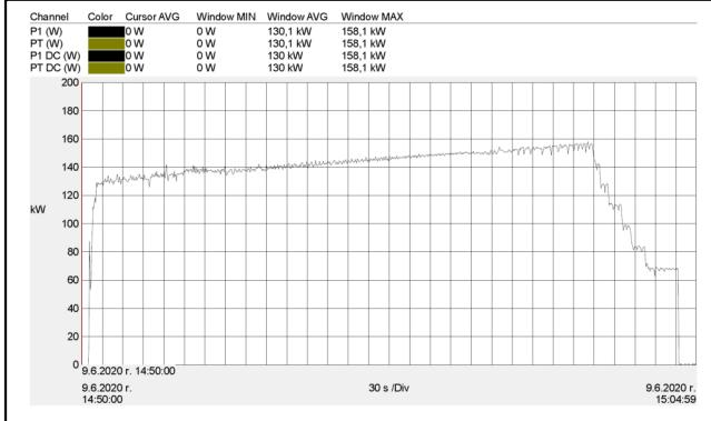
Fig. 4. Downstream DC power.
