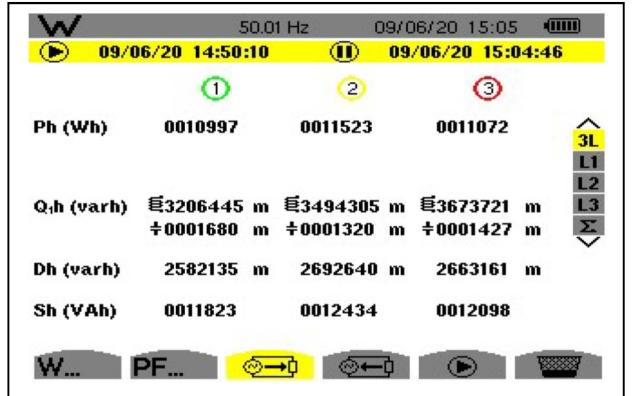
Fig. 9. Upstream AC Energy phase by phase.
