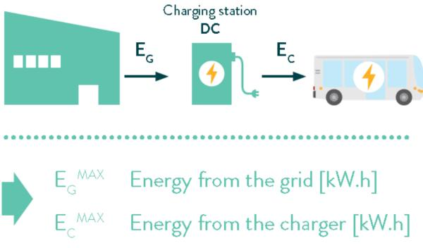
Fig. 1. Usable Energy Content. (Source E-SORT [2])
