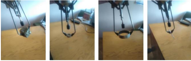
Fig. 2. Gropper grasping different objects: stone, rolling element bearing, bushing, pen.
