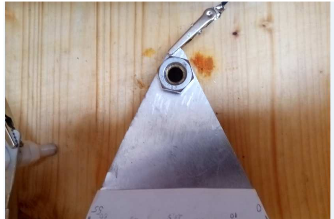
Fig. 2. Connection between the aluminum plate and the wooden box
