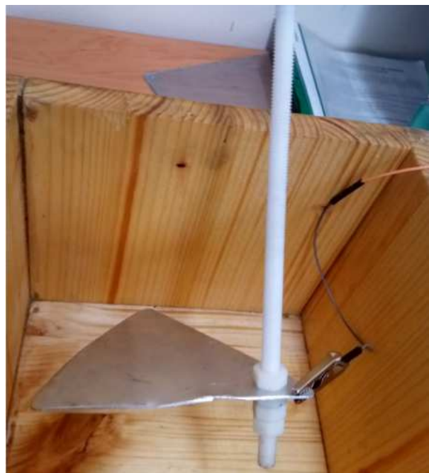
Fig. 3. Plastic rod connected to an aluminum plate
