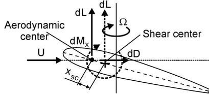
Fig.5. Section moment relevant geometry of a blade element
