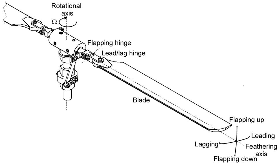
Fig.1. Sketch of pattern rotor with flapping and lead/lag hinges
