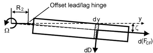
Fig.4. Blade aerodynamic and centrifugal forces about the lead/lag hinge
