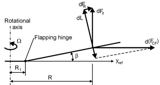
Fig.3. Blade aerodynamic and centrifugal forces about the flapping hinge
