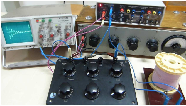
Fig. 14 The transient in RLC circuit
