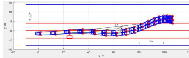
Fig. 7. Graphical measurement of the turning radius.
