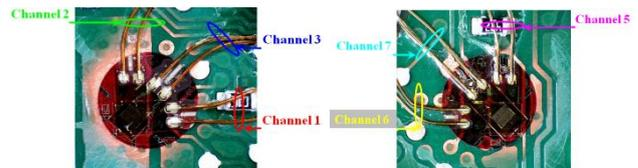
Fig. 8. Experimental panel with located sensors
