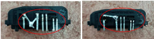
Fig. 5. Leak check samples at 1000 V
