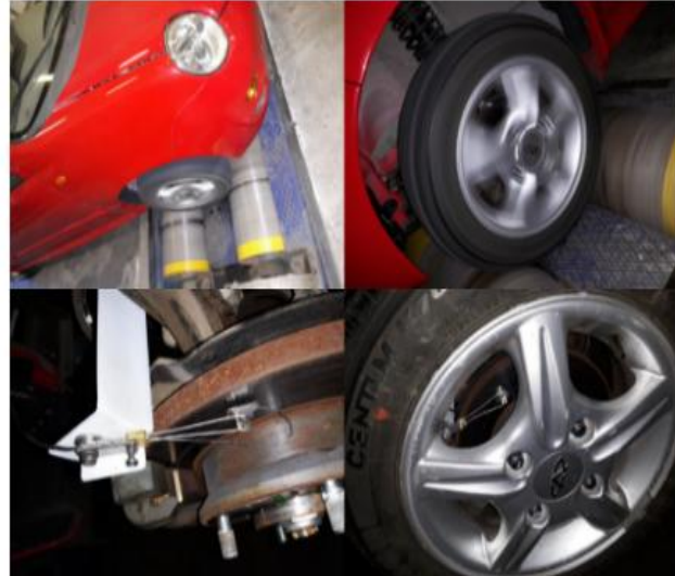
Figure 10. Location of the brake disc thermocouple and of the vehicle on a dynamometer stand.
