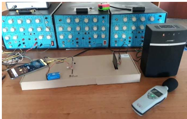
Fig. 7. Conducting an experiment using a infrared LED as a source of optical radiation
