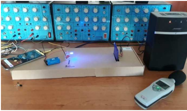
Fig. 5. Conducting an experiment using a blue LED as a source of optical radiation
