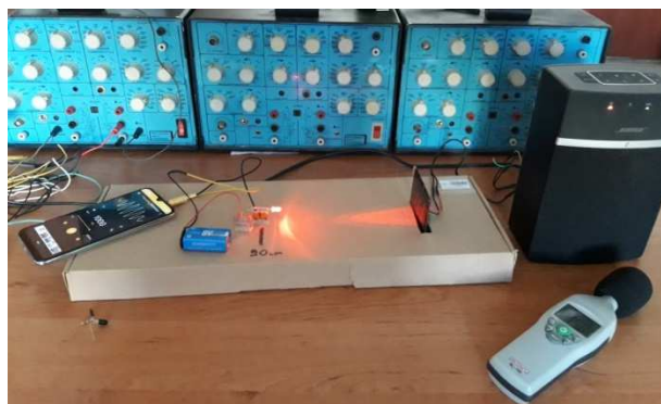
Fig. 7. Conducting an experiment using a infrared LED as a source of optical radiation
