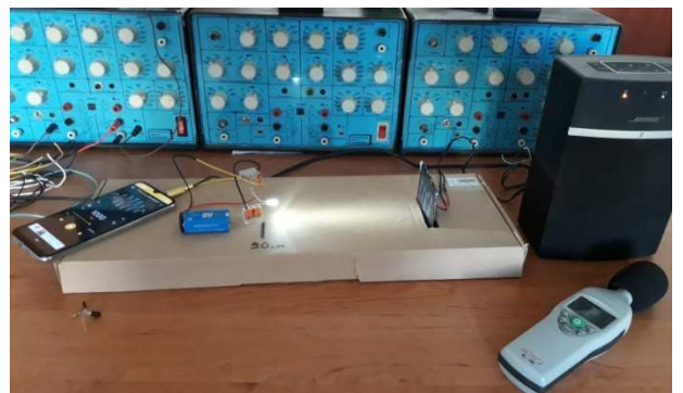
Fig. 4. Conducting an experiment using a white LED as a source of optical radiation
