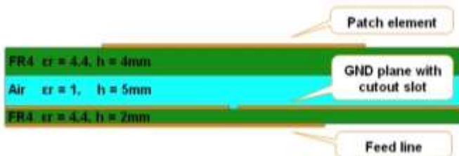
Fig. 4 Proposed aperture-coupled microstrip antenna stack-up
