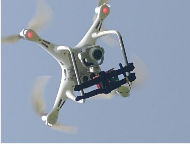
Fig. 1. DJI Phantom 3 drone with mounted boards with Melexis MLX90640 sensor during the flight
