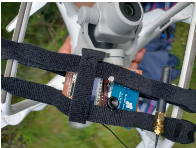
Fig. 2. DJI Phantom 3 drone with mounted boards with Melexis MLX90640 sensor close look
