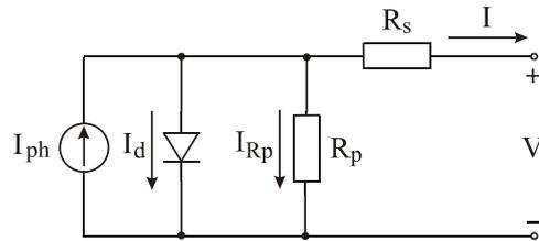
Fig. 1. Equivalent circuit of PV module
