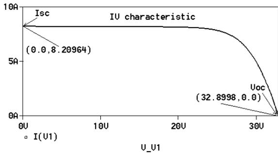
Fig. 7. Simulated IV characteristic
