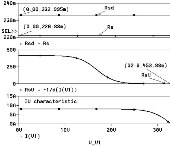
Fig. 5. Determination of  $R_s$
