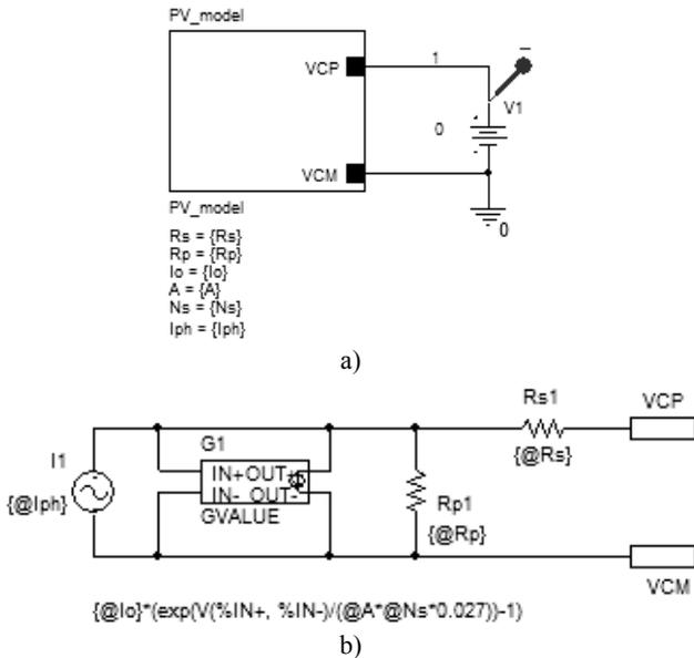
Fig. 6. PSpice macromodel of the PV module defined as a block (a) and parameterized subcircuit (b)
