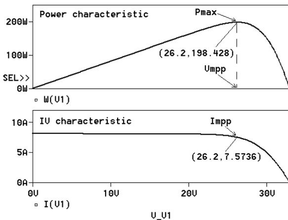
Fig. 8. Simulated power characteristic
