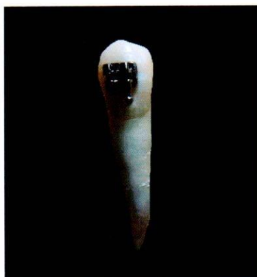
Fig. 1. Bracket bonded on a molar (prepared for experimental analysis)
