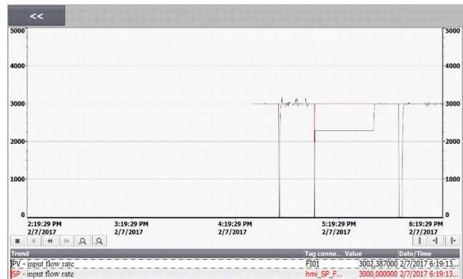
Fig. 7. PI regulator controlling the input flow-rate
