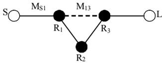
Fig.2. Coupling scheme of an asymmetric three pole filter
