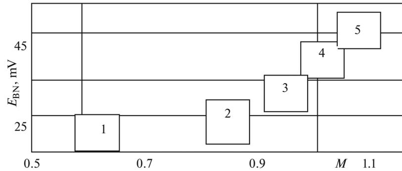
Fig. 4. Characteristic areas in two-parameter non-destructive testing of cast iron. Information parameters:  $E_{BN}$  and  $M$ .
