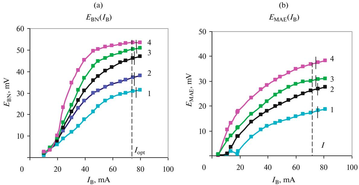
Fig. 2. One-parameter confidence intervals of the  $E_{BN}(I_B)$  and  $E_{MAE}(I_B)$  series of curves of the groups of comparative samples of 40X steel.
