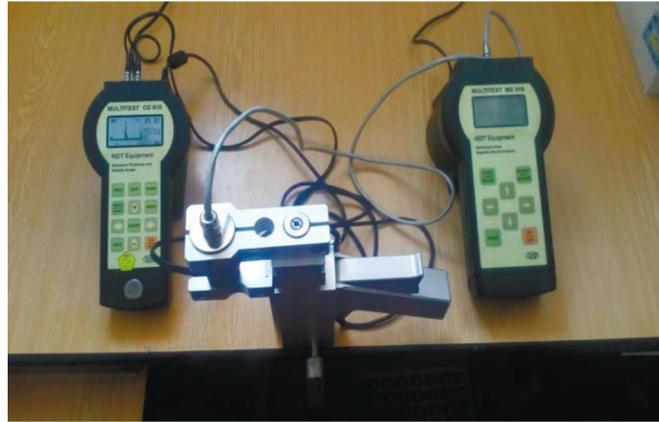
**Fig. 1.** Appearance of the system with configuration—test pliers DK100 and devices MULTITEST-MC010 and MULTITEST-CD010.
