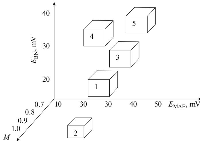
Fig. 5. Characteristic areas in three-parameter non-destructive testing of cast irons Information parameters,  $M$ ,  $E_{BN}$  and  $M_{AE}$ .
