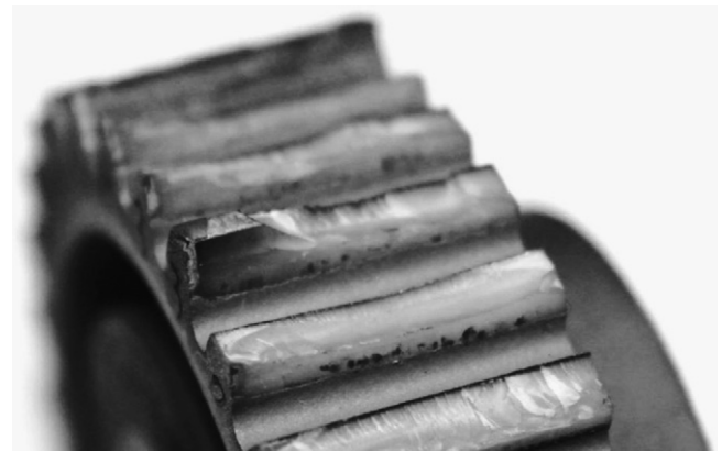
Fig. 8. Pitch line fracture in a boron nitride coated PA gear run in mesh with a steel gear.
