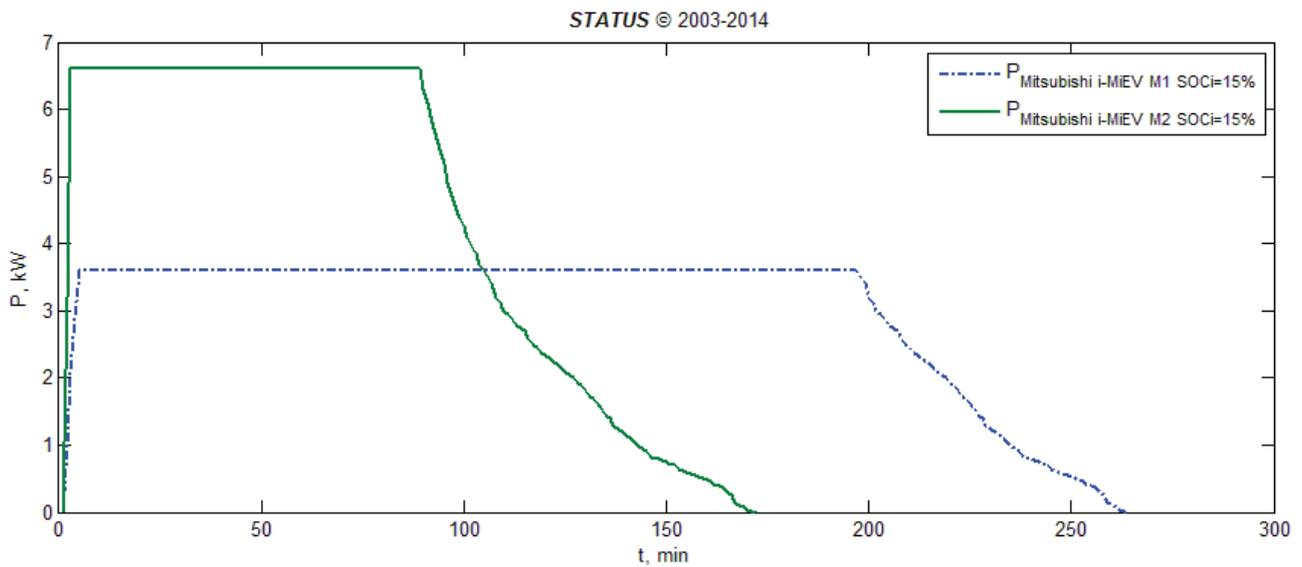
**Fig.2.** Load profiles of 3,6kW Mode 1 and a 6,6kW Mode 2 charging.
