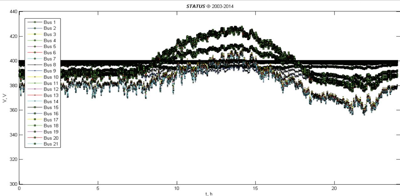
**Fig.7.** Voltage profile evolution without EV charging (Scenario 1).
