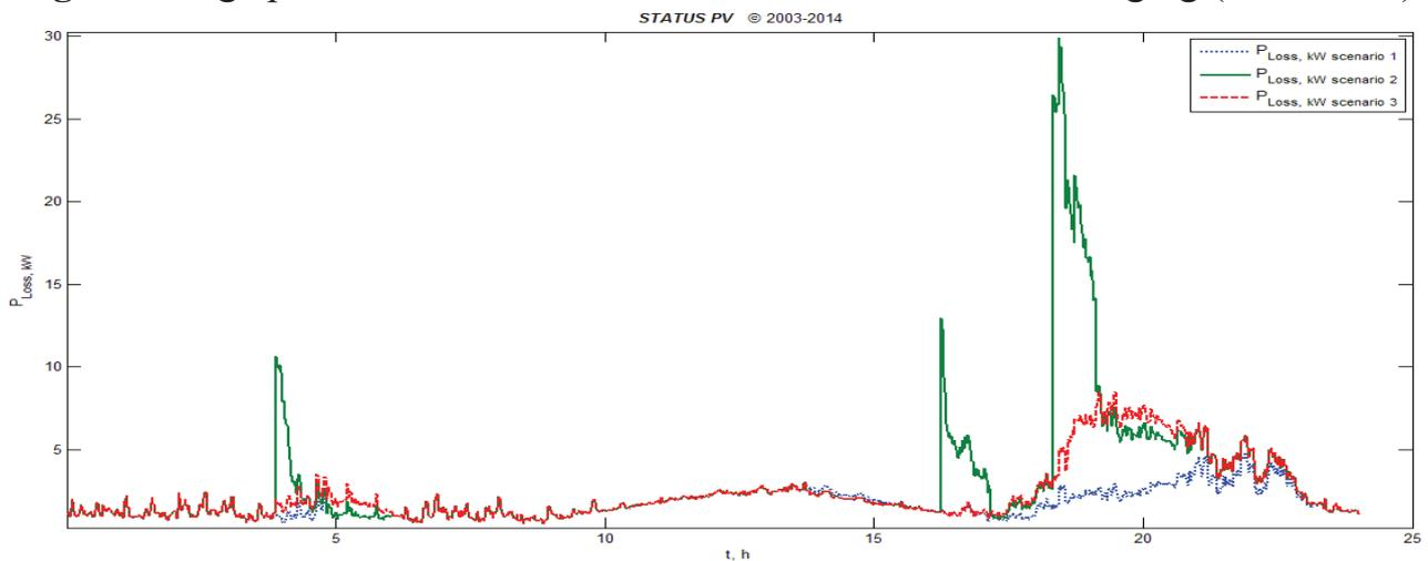
**Fig.10.** Aggregated power losses evolution during Scenario 1, 2 and 3.
