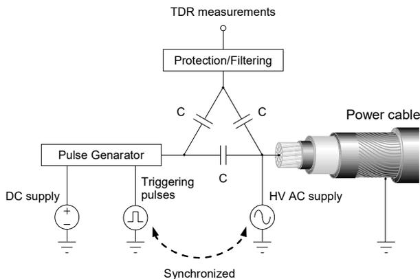
Fig. 6. Measurement system for performing TDR phase-locked to the applied high voltage.
