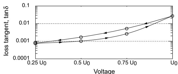
Fig. 4.  $\tan\delta$  measurements on a water treed cable at voltages up to the service voltage  $U_0$  at 1 Hz. The observed voltage dependence of the loss tangent confirms the effect of water treering. By repeating, subsequently, the measurements at identical voltage levels one observes a hysteresis type of effect that is indicative for significantly deteriorated insulation.
