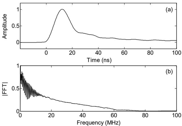
Fig. 7. The pulse generator signal output (a) and frequency content (b).
