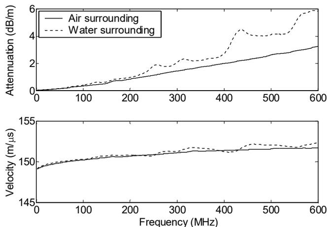
Fig. 3. Measurements of the attenuation constant ( $\alpha$ ) and velocity ( $v$ ) conducted when air and water are surrounding the MV power cable.
