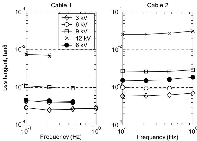
Fig. 10.  $\tan\delta$  for Cables 1 and 2. Significant voltage dependency can be observed in both cases which is indicative of water tree ageing.
