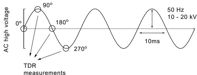
Fig. 5. TDR measurements performed while applying AC high voltages.
