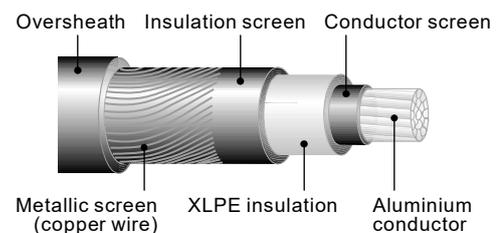
Fig. 1. MV power cable design.
