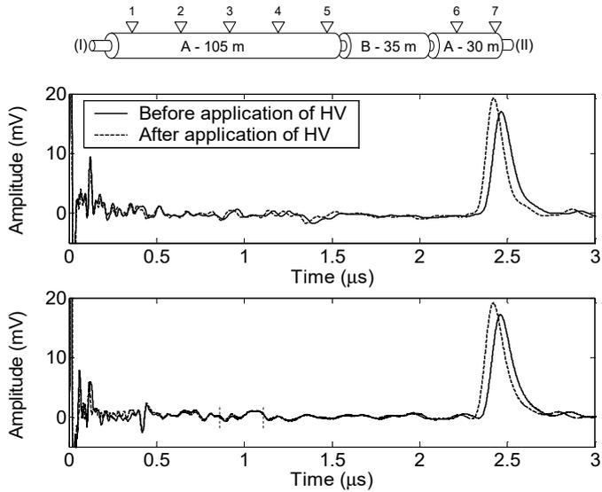
Fig. 9. TDR measurements from both sides (Cable 2).
