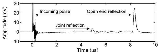
Fig. 2. Example of multiple reflections in TDR measurements on distribution class power cables.
