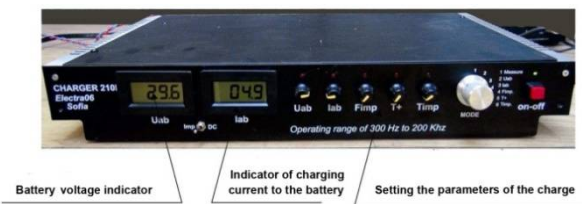
Fig.3 Charger with indicators and control
