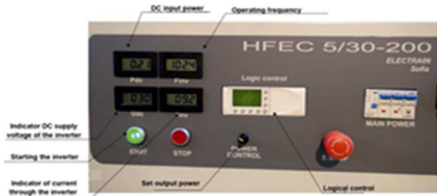
Fig.2 Inverter with indicators and control
