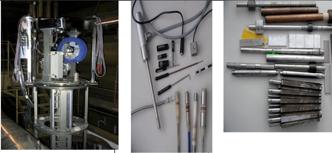
Fig. 29. Testing tools for the ET process (left to right: handling device, probes and reference pieces - tubes with implanted flaws used for tuning the signal)
