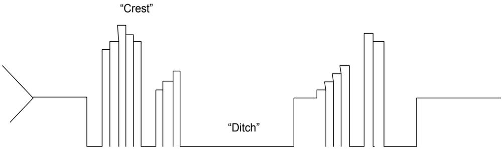
Fig. 13. Slip planes in material fatigue
