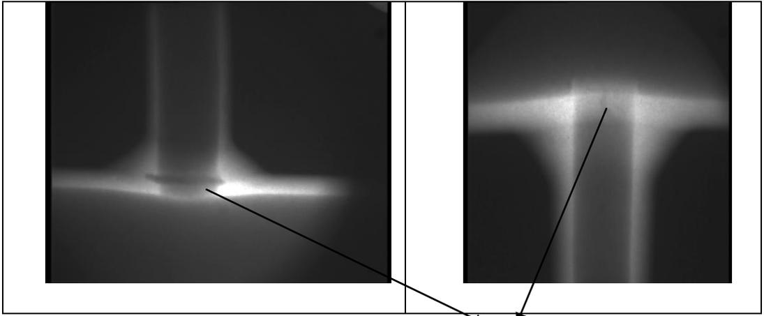
Fig. 32. Results from radiographic testing - discontinuities in metal are visible
