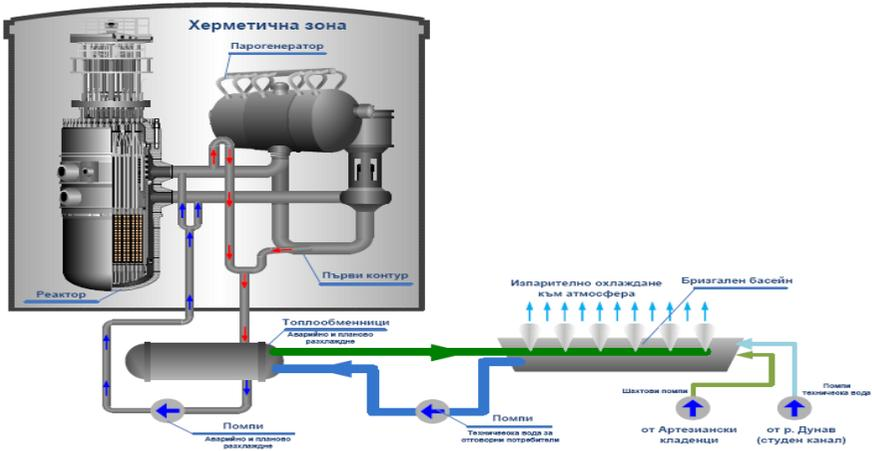
Fig.19. Nuclear reactor unit, type WWER-1000
