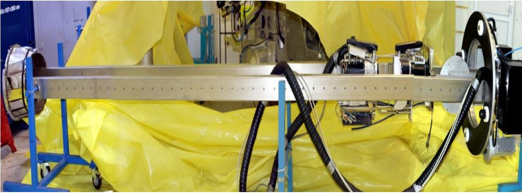
Fig. 28. Handling device for automated eddy current testing
