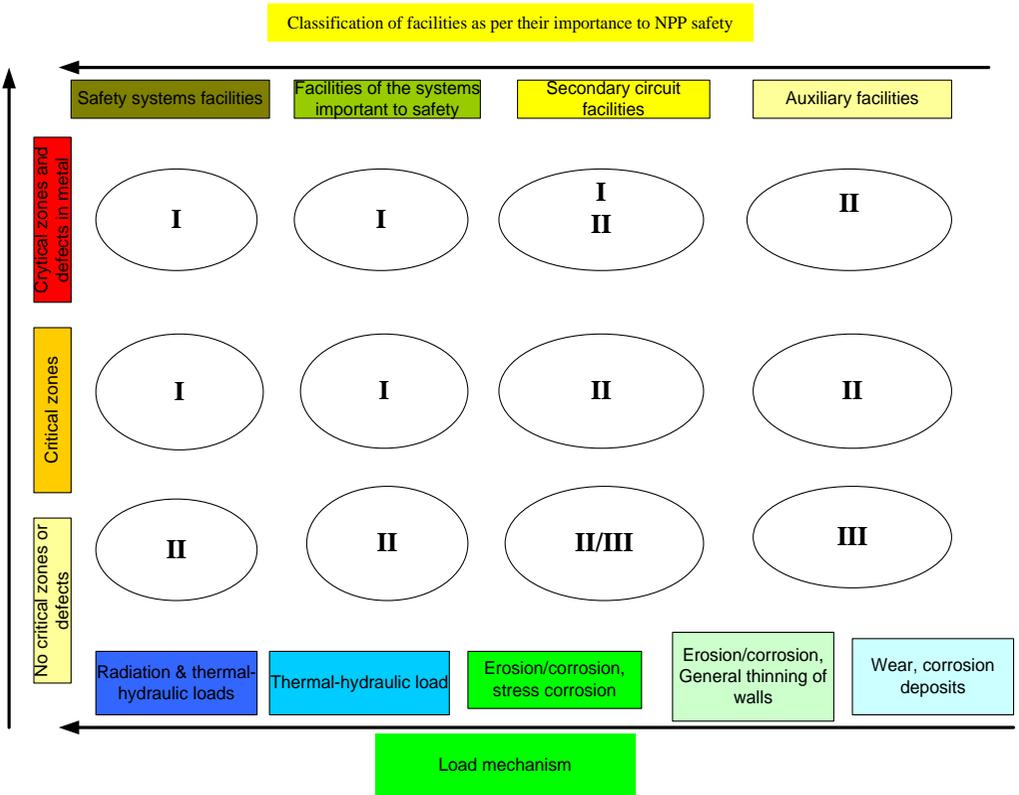
Fig. 50. Categorisation of inspection according to the importance of facilities for the safe plant operation and the loading mechanisms
