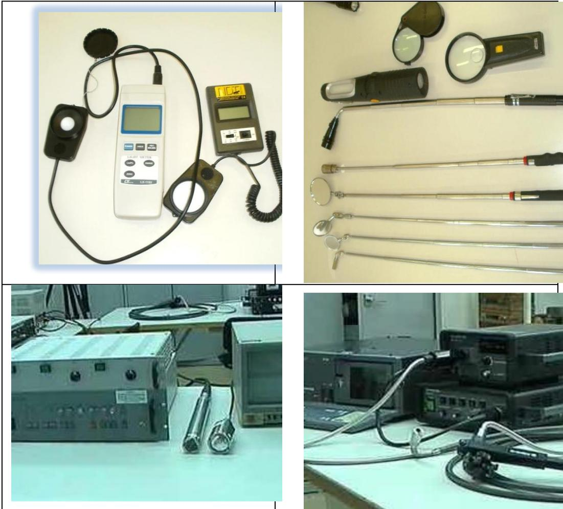
Fig. 24. Visual testing technical tools; magnifying glasses (above), boroscopes and endoscopes (below)
