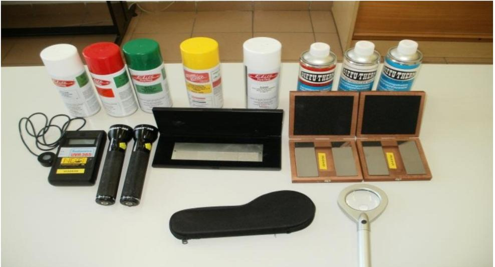
Fig. 27 Technical tools for inspection with penetrant liquids - penetrants (the kit consists of penetrating, washing and developing liquids)
