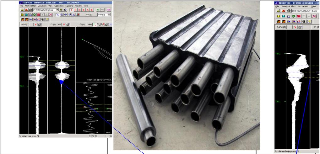
In the left, there is the probe signal from the end of the tube (end-off effect); in the right is the eddy current signal from a hole in the tube wall (100% wear of the tube wall).
