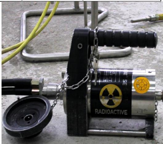
Gamma flaw-detector using a selenium (Se) source
