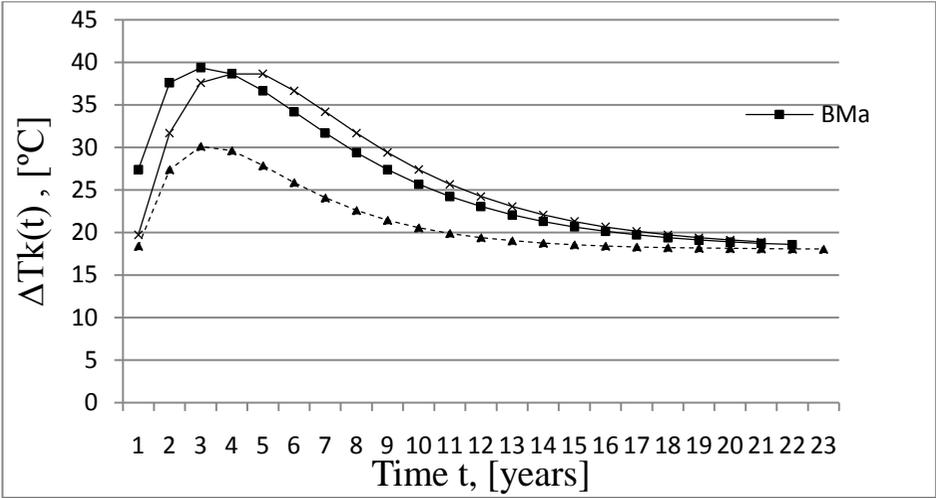
Fig. 10. Thermal ageing: dependency of  $\Delta T_K(t)$  on time  $t$  (or thermal induced part of  $\Delta T_K$ ) for BM and WM
