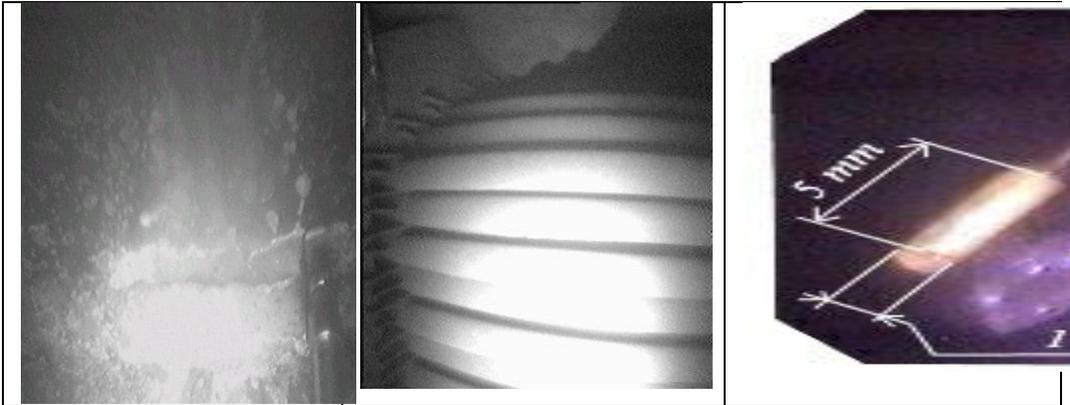
Fig. 26. Visual testing and measurement inspection of vessel interior surfaces
