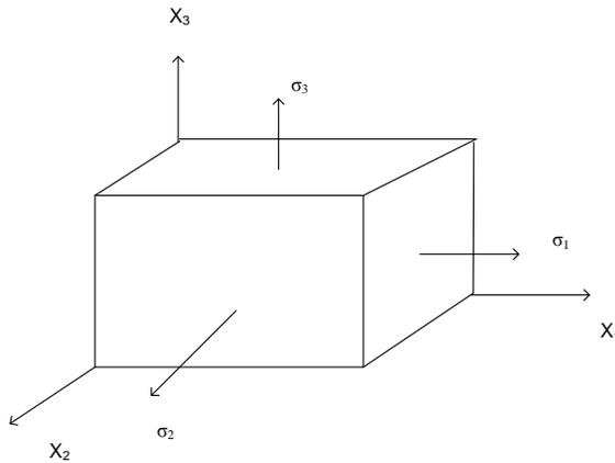
Fig. 3. Forces acting along the three main planes of the stress tensor
