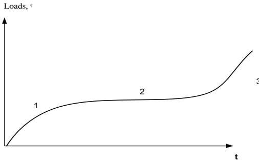
Fig.17. Section 1 – undetected creep; Section 2 – constant speed creep; Section 3 – increasing speed creep, terminating with fracture
