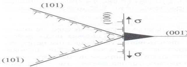
Fig. 5. The Cottrell model of crack formation; 101 - slip planes of dislocations; 100 - plane of forming of new dislocations; 001 - plane of crack formation
