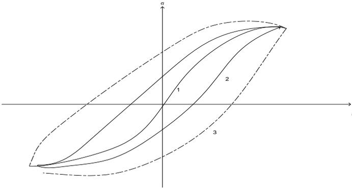
Fig. 16. Diagram  $\sigma - \epsilon$  for repeated monotonous loading (1); during cyclic loading (2); curve envelope (3)
