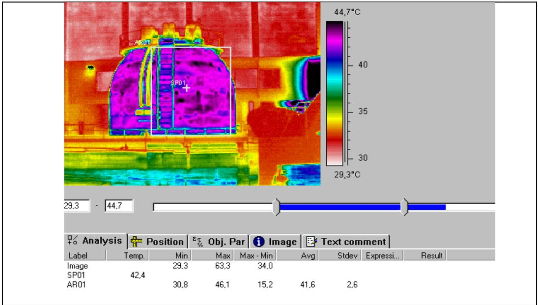
Fig. 34. A photo and thermograms of mechanical pieces of equipment. (top images - a pump; bottom one - reactor pressure vessel)
