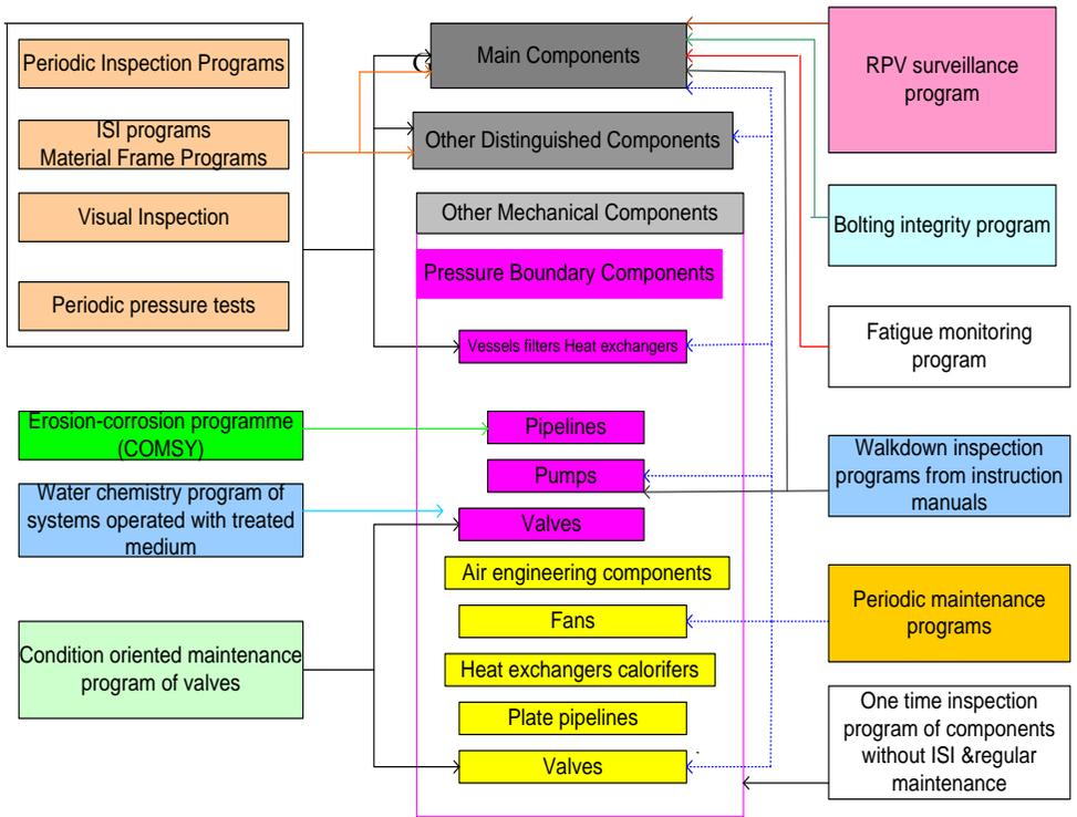
Fig. 23. Inspection programmes for NPP facilities
