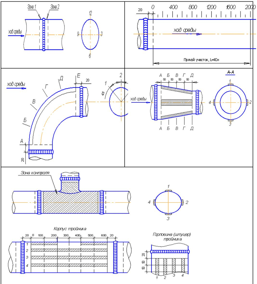
Fig. 37. Thickness inspection measurements of a pipe, a bended section, and a T-joint (inspection schemes)
