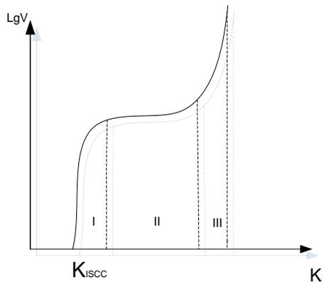
Fig. 6. Diagram of the static stress corrosion cracking toughness
