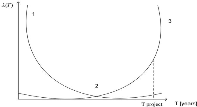
Fig. 2. Dependence of the failure rate function  $\lambda(T)$  on the operation time period  $T$ , 1 – failures due to equipment adjustments and installation; 2 – design operational life; 3 - failures resulting from degradation of the mechanical properties of metal
