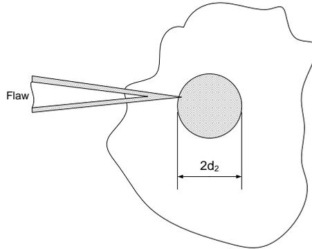
Fig. 7. Material embrittlement around the crack peak
