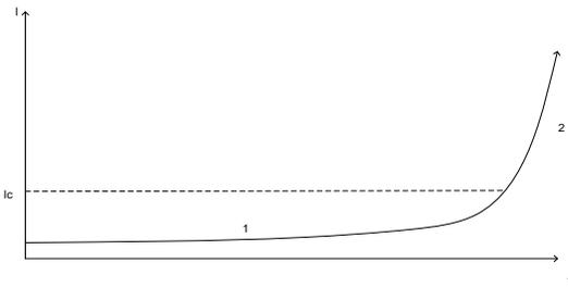
Fig. 14. Progress of the crack length  $l$  within the time period  $t$ .
