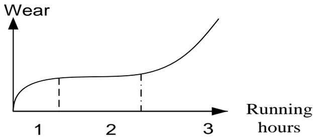
Fig. 18. Wear depending on the hours in operation
