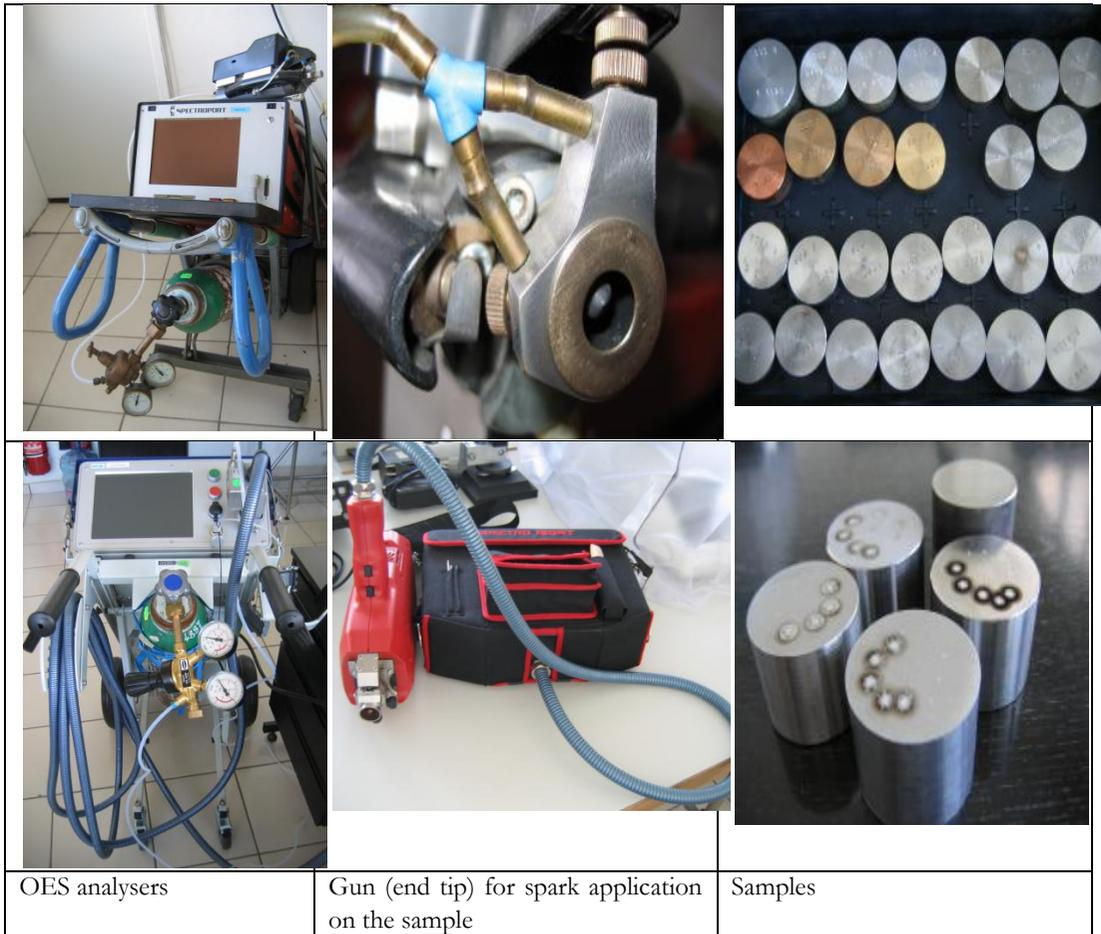
Fig. 44. Technical instruments for the spectral testing method
