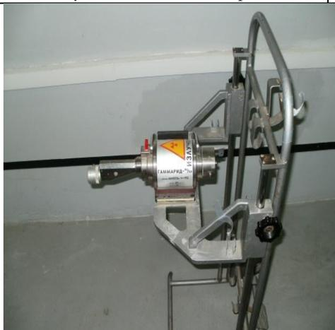
Gamma flaw-detector with an iridium (Ir) source
