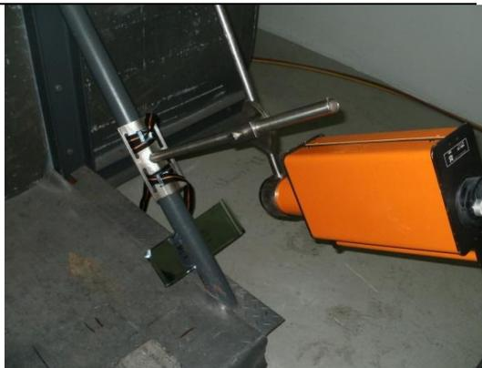
X-ray instrument - X-ray tube and collimator
