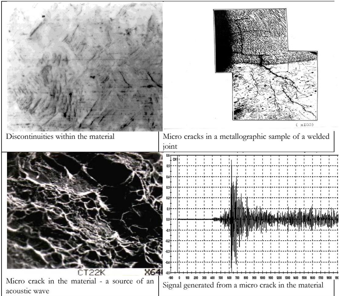
Fig. 45. Acoustic emission method of testing (examination)
