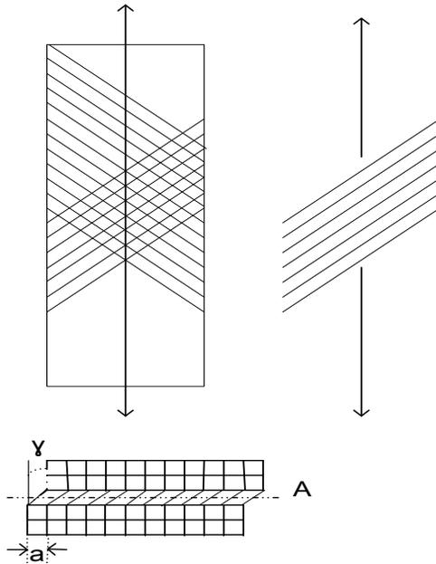
Fig. 4. Slip plane (A), the smallest plastic deformation corresponding to the slip of one element (a)
