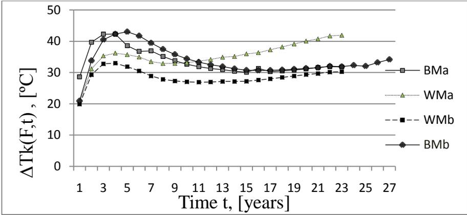
Fig. 11 General ageing (neutron+thermal) dependency of  $\Delta T_K(F,t)$  on time  $t$  for BM and WM
