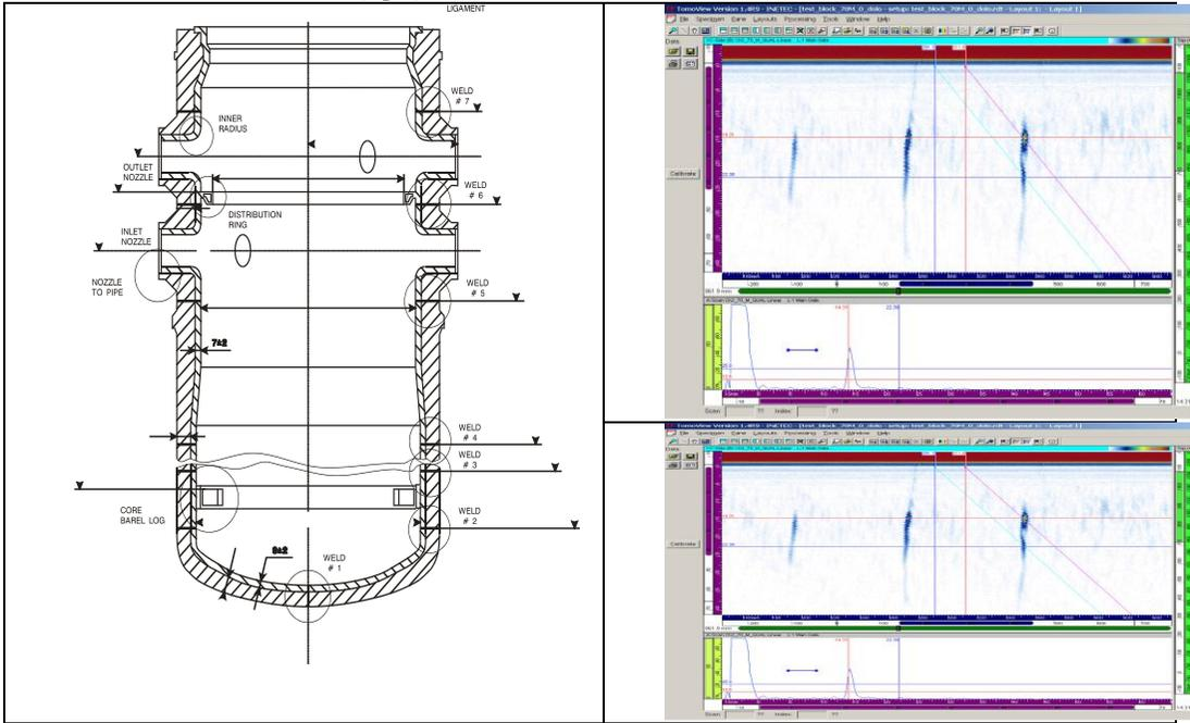
Fig. 36. Ultrasonic testing of a reactor pressure vessel - a schematic view of a nuclear reactor (left) and results from UT (right)
