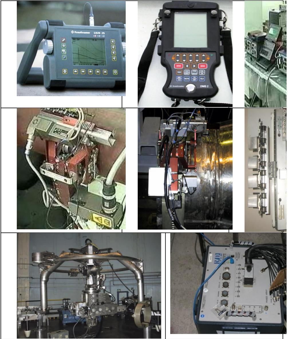
Fig. 35. Ultrasonic flaw detectors and automated ultrasonic testing systems
