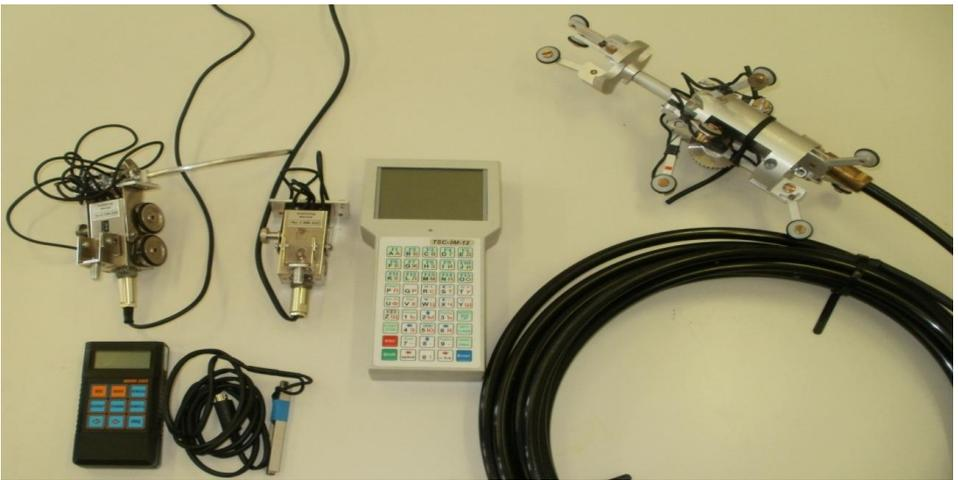
Fig. 41. Technical devices used by the metal magnetic memory testing method
