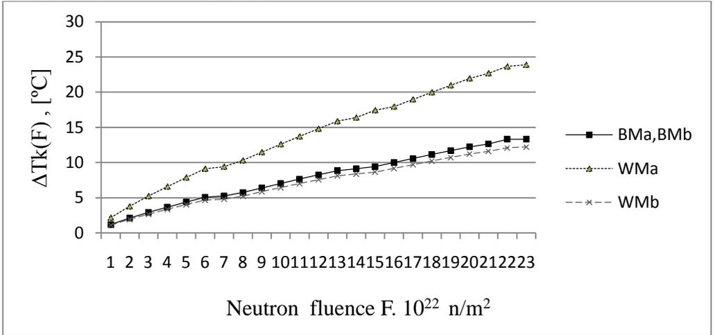
Fig. 9. Neutron ageing - dependency of  $\Delta T_K(F)$  on fluence  $F$  for BM and WM, or a neutron induced part of  $\Delta T_K(F, t)$
