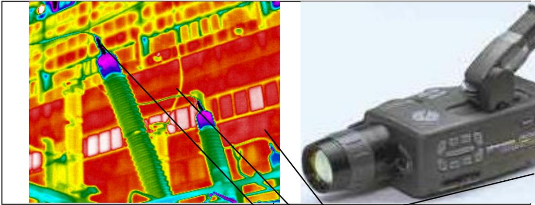
Fig. 33. Thermograms of electrical equipment - elevated thermal emissivity is observed for the voltage inputs; thermal imaging camera
