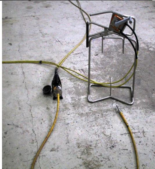
Collimators and hoses for gamma flaw-detectors
