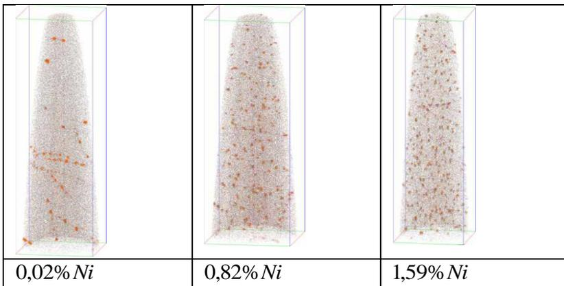
Fig. 8. Formation of dislocations in samples of varying weight percentage of Ni ( $0,22Cu - xNi - 1,6Mn$ ) at temperature of  $T = 290 \div 310^{\circ}C$
