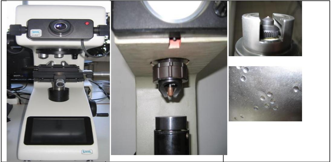
Fig. 43. Hardness meters, indenter footprints on the surface of the tested object (the last one, left)
