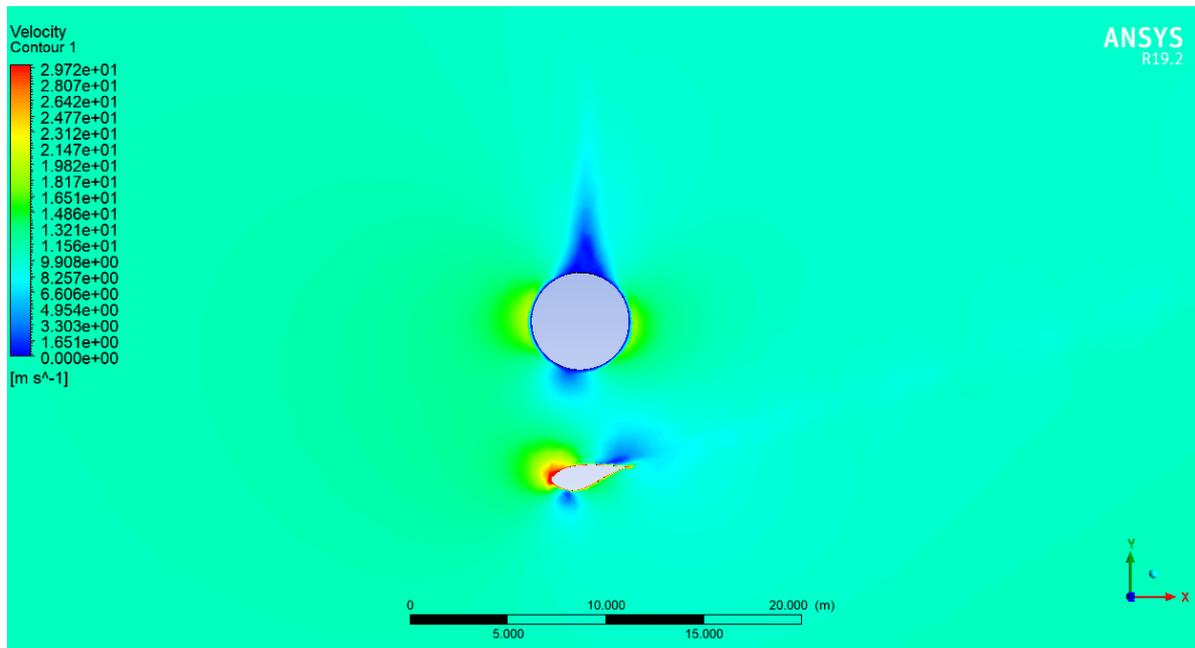
**Figure 7.** Velocity field of DU30 passing in front of the tower.
