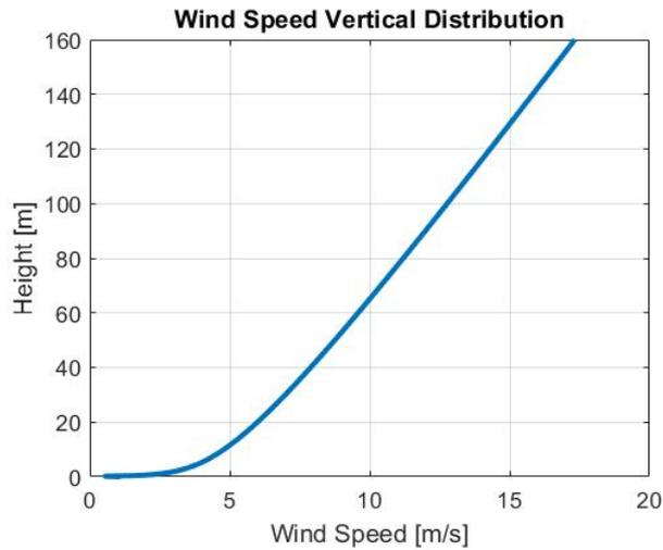
**Figure 3.** Wind speed vertical distribution.
