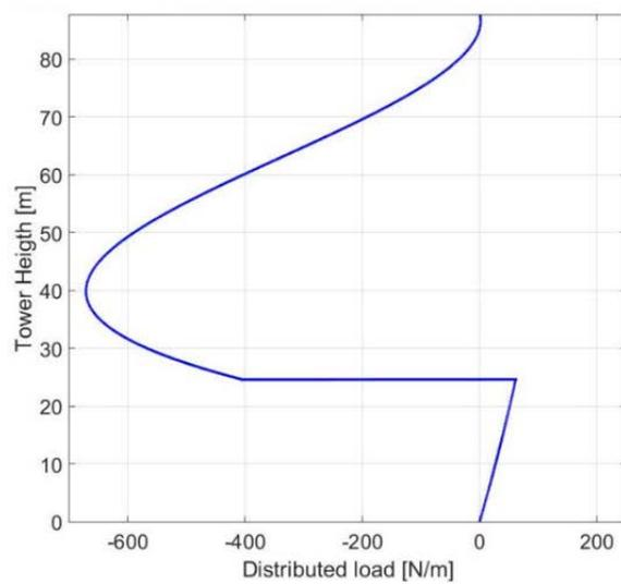
**Figure 14.** Tower drag force distribution with shading.
