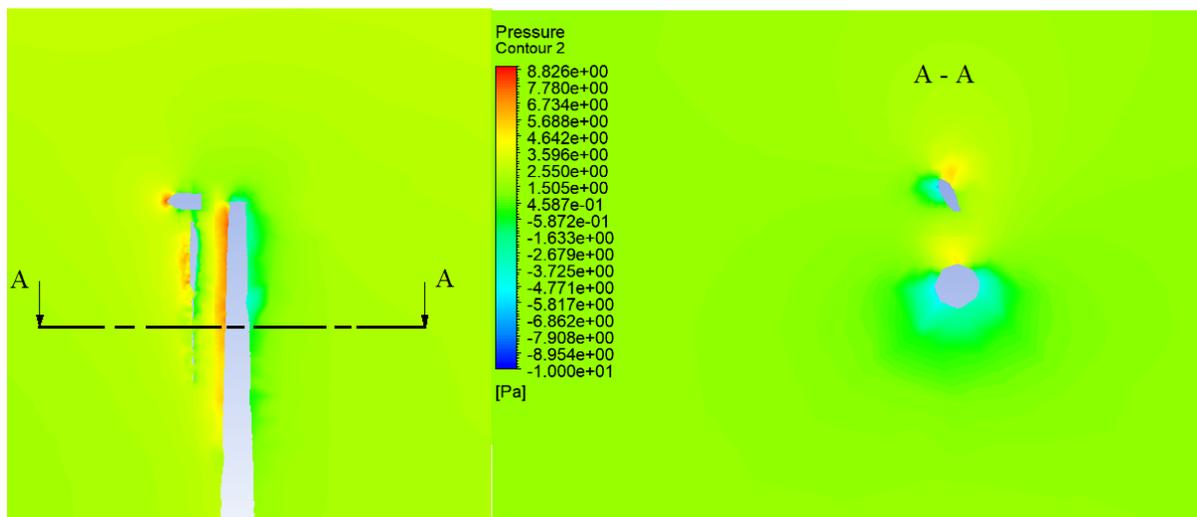
**Figure 2.** Pressure field deviation between the blade and the tower of an arbitrary wind turbine generator with horizontal axis caused by shading.
