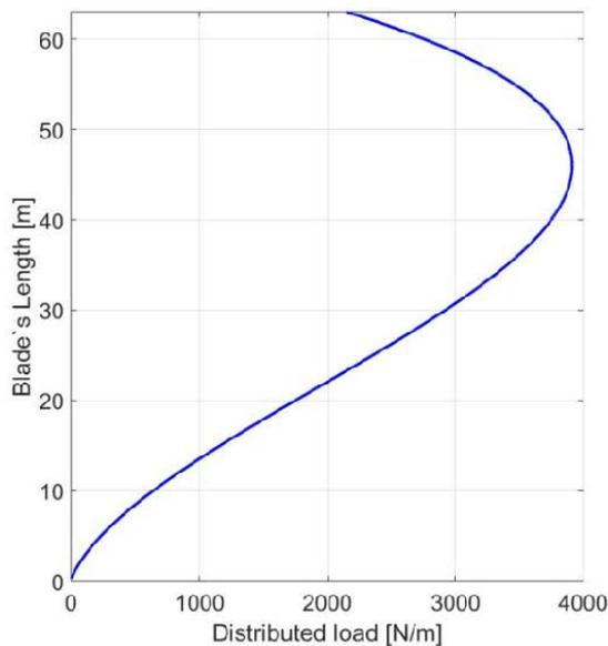
**Figure 15.** Blade thrust force distribution without shading effects.
