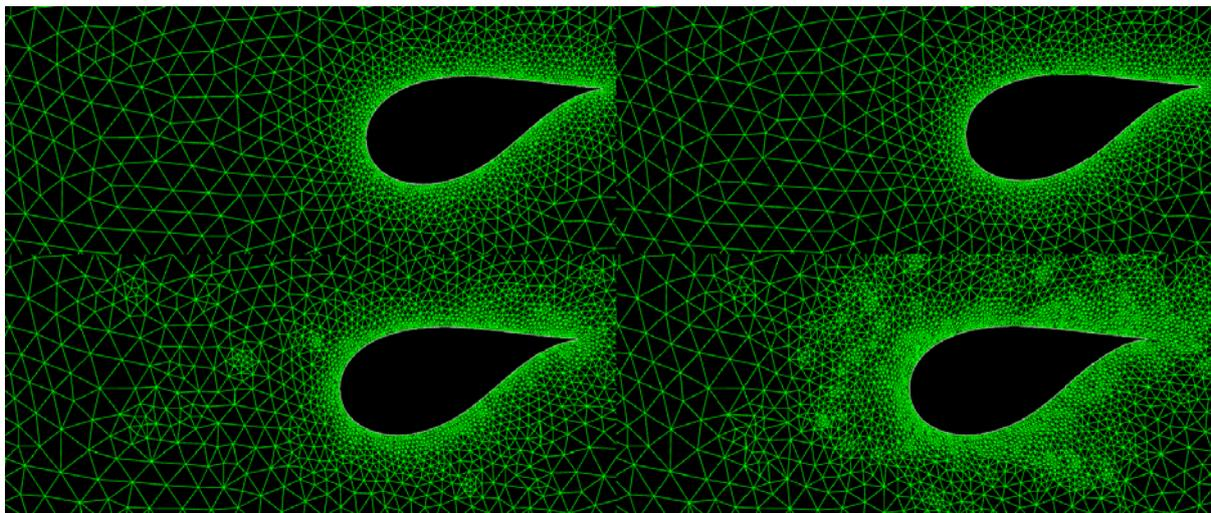
**Figure 5.** Dynamic mesh of the DU40 airfoil simulation for 1st, 3rd, 5th and 10th time steps of the calculation.
