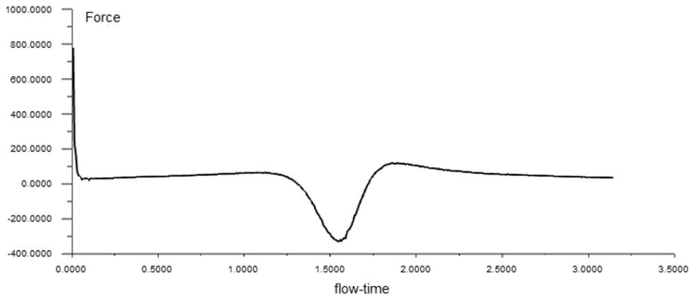
**Figure 9.** Tower drag force as a function of time.
