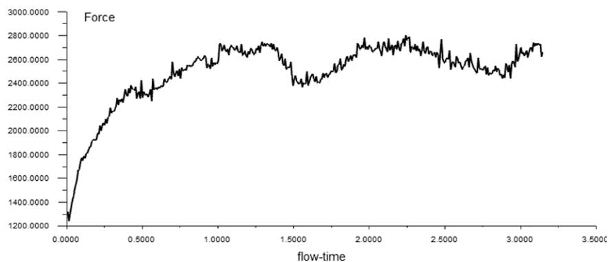
**Figure 11.** DU30 thrust force change in time.
