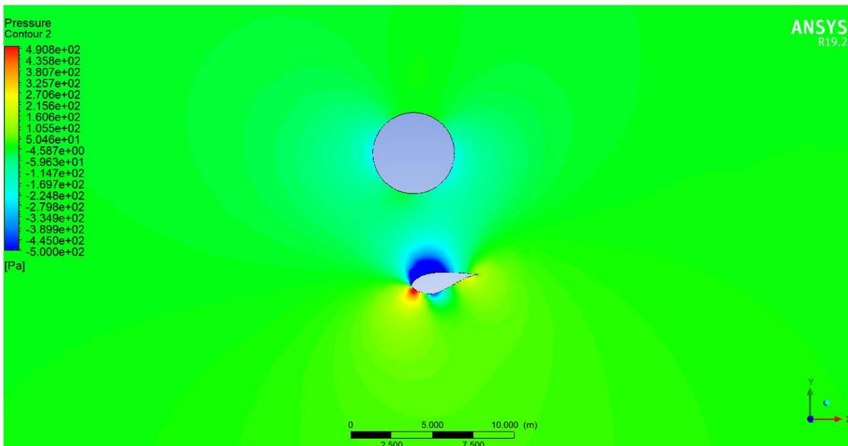
**Figure 8.** Pressure field of DU30 passing in front of the tower.
