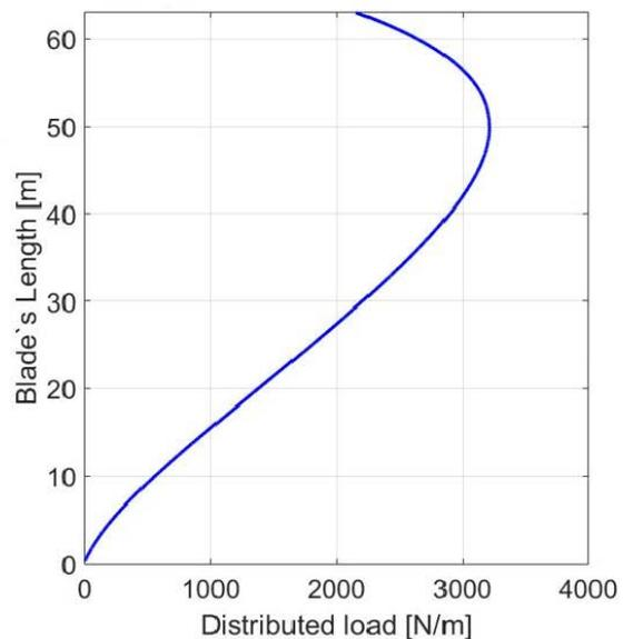
**Figure 16.** Blade thrust force distribution with shading.
