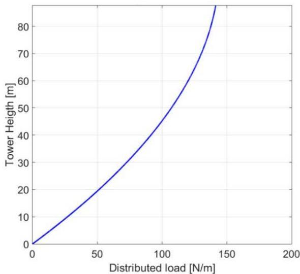
**Figure 13.** Tower drag force distribution without shading effects.
