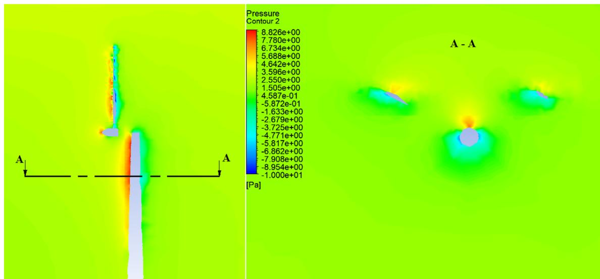
**Figure 1.** Pressure field distribution around the blade and the tower of an arbitrary wind turbine generator with horizontal axis.
