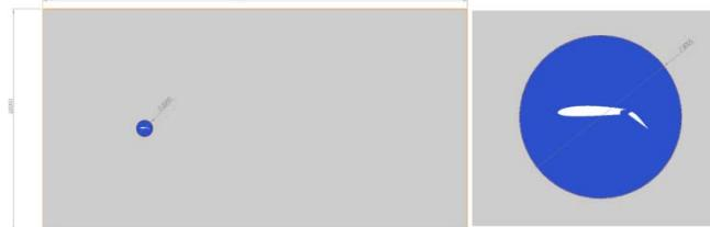
Fig. 3 2D plane model of NACA 2412 a slotted flap with gap size 10% of the main chord and angle of deflection 40°
