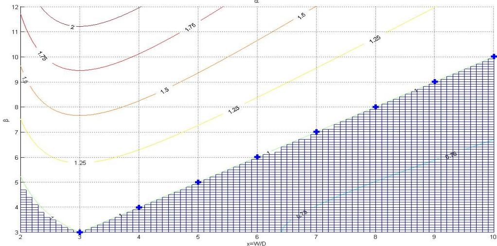
Fig. 3. Evolution of  $\alpha$  as a function of  $x$  and  $\beta$ , for single airgap.
