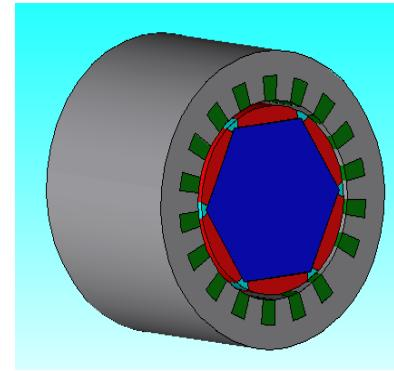
Fig. 1. Radial-flux permanent-magnet machine
