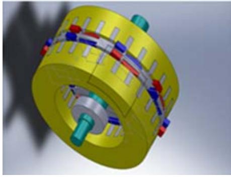
Fig. 2. Axial-flux permanent-magnet machine
