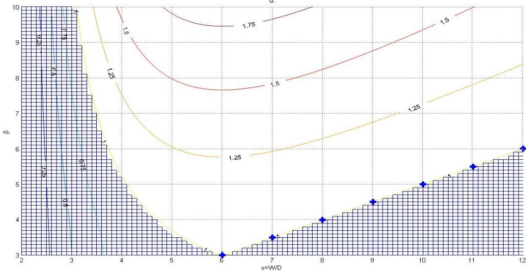
Fig. 4. Evolution of  $\alpha$  as a function of  $x$  and  $\beta$ , for double airgap.
