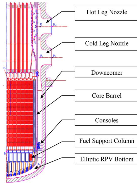
FIGURE 1. Reactor vessel and internals of Kozloduy-6
