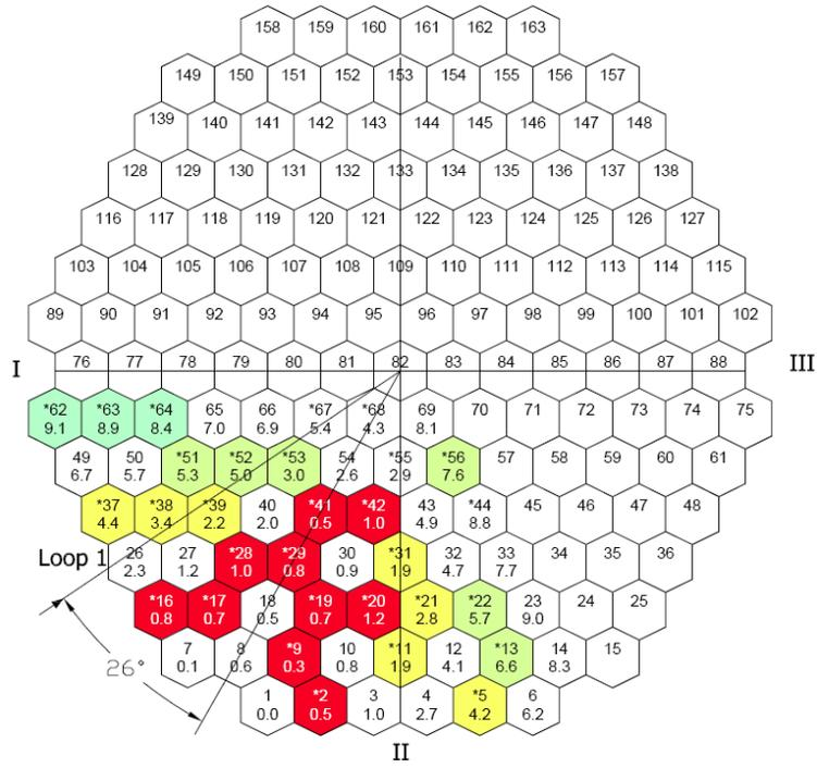
FIGURE 3. Plant data: estimated temperature differences from cold leg to assembly inlets, and angular turn of loop#1 flow center in the final state. Here  $dT_k = T_{\text{cold leg}1} - T_k$ ,  $k=1,163$
