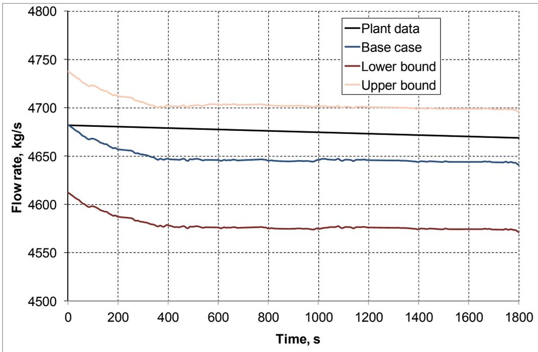
FIGURE 12. Time history of mass-flow rate in hot leg nozzle #3
