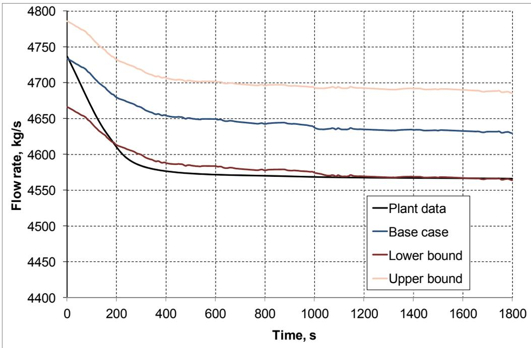
FIGURE 10. Time history of mass-flow rate in hot leg nozzle #1
