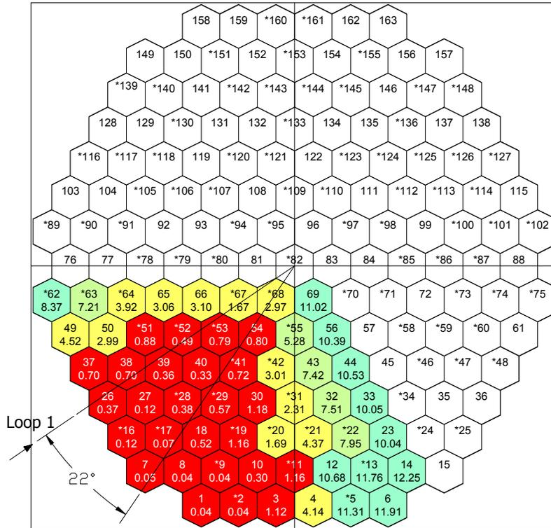
FIGURE 5. RELAP 24-sector vessel model: Computed disturbed sector and angular turn of loop#1 flow center in the final state
