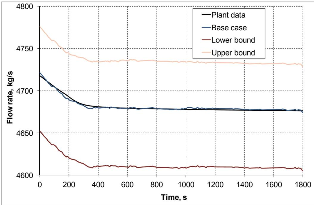
FIGURE 11. Time history of mass-flow rate in hot leg nozzle #2
