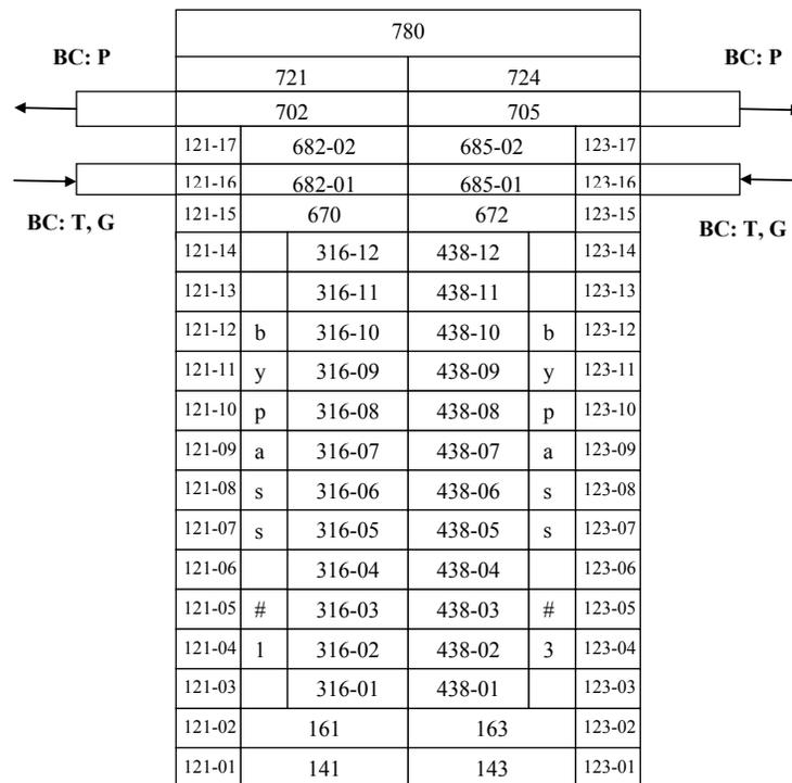
FIGURE 2. 12 sector models: Axial discretization scheme
