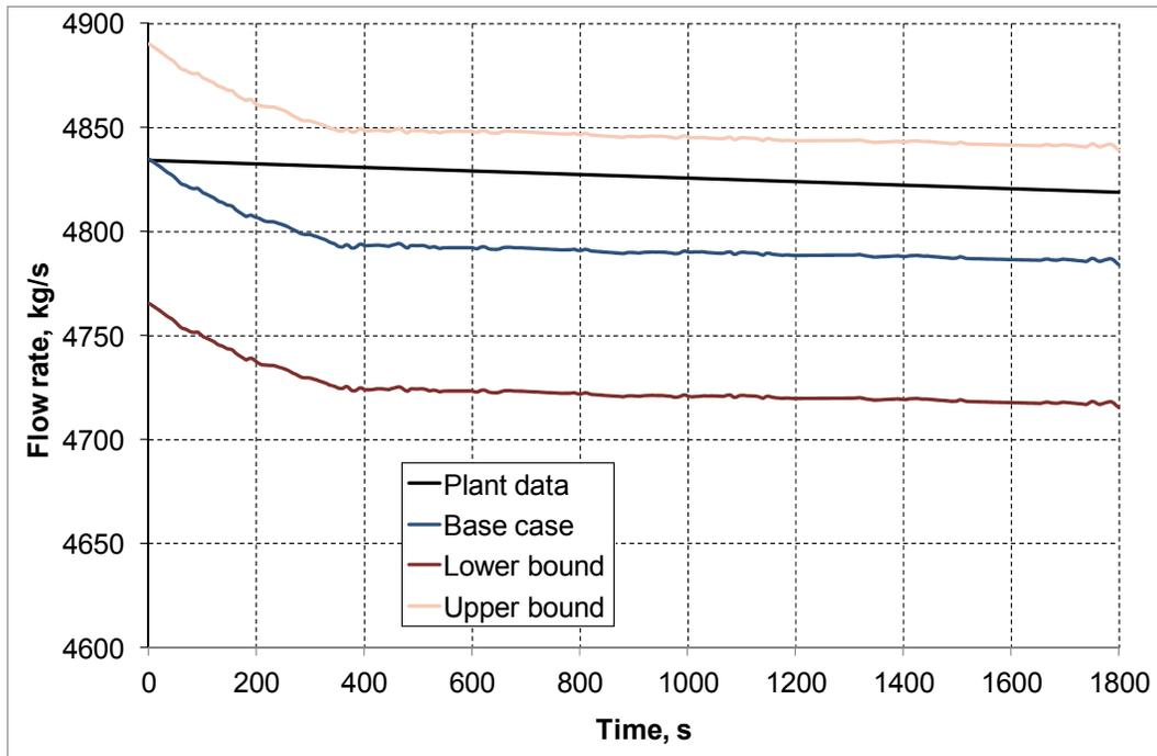
FIGURE 13. Time history of mass-flow rate in hot leg nozzle #4
