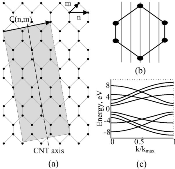
FIG. 2 (A) CARBON NANOTUBE WITH CHIRALITY VECTOR  $C(2,1)$  OVERLAID ON GRAPHENE ATOMIC LATTICE; (B) GRAPHENE BRILLOUIN ZONE AND CNT DISCRETIZATION LINES; (C) ENERGY LEVELS OF A  $C(5,0)$  CNT CALCULATED BY THE TIGHT-BINDING MODEL APPROXIMATION.
