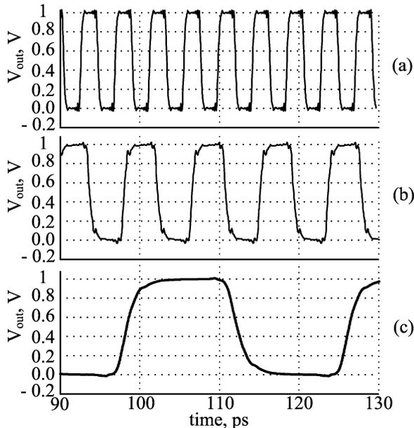
FIG. 8 TRANSIENT RESPONSE OF 7-STAGE RING OSCILLATOR CIRCUIT USING CNTFETs. (A) WITHOUT ANY PARASITIC CAPACITANCES, (B)  $C_{g-sub}$  AND  $C_{g-sd}$  ARE ADDED, (C) ALL PARASITIC CAPACITANCES FROM FIG. 7 ARE ACCOUNTED FOR.
