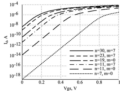
FIG. 6 TRANSFER CHARACTERISTICS OF CNTFETs WITH DIFFERENT CHIRALITIES AT  $V_{DS} = 0.9$  V
