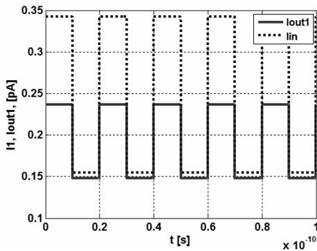
Fig. 19 First output and input current versus time
