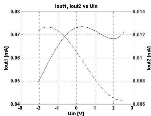
Fig. 9 The output characteristics of the microelectronic circuit, analogous to the network M2
