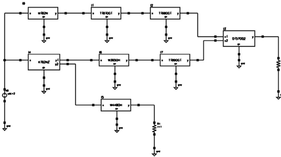
Fig. 6 Microelectronic circuit analogous to HBN coded in Cadence
