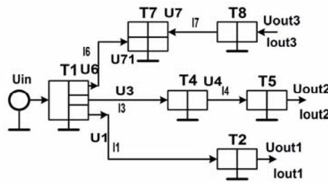
Fig. 7 Functionally analogous to HBN M4 microelectronic circuit consisting of block-elements coded in Matlab
