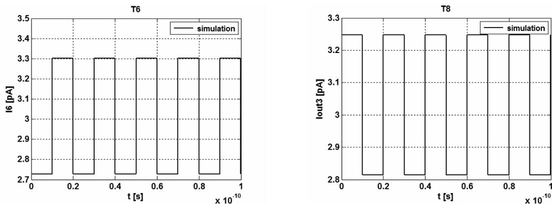
Fig. 27  $I_{in3}$  ( $I_6$ ) Input and output currents for the third output of the circuit versus time
