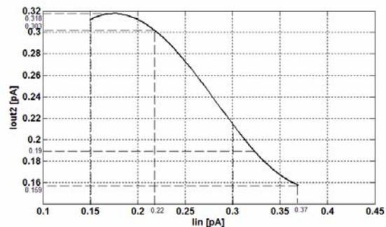
Fig. 17 Transfer characteristic of the second output of the circuit. The output current as a function of the input current.
