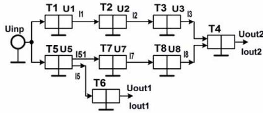
Fig. 5 Microelectronic circuit analogous to HBN coded in Matlab
