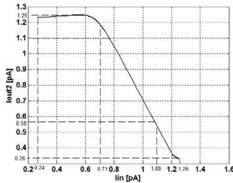
Fig. 22 Transfer characteristic of the second output of the circuit
