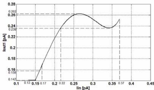
Fig. 16 Transfer characteristic of the first output of the circuit. The output current as a function of the input current.
