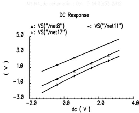
Fig. 12 Outputs voltages vs. input voltage in Cadence
