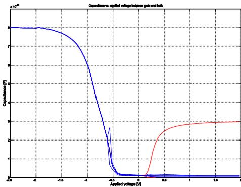
Figure 4. Fitting C-V curves by changing variables  $B_1$  (blue) and  $B_2$  (red) in inversion and depletion regions.
