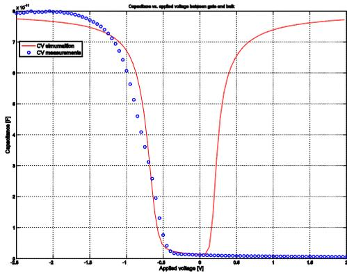
Figure 2. Simulation of C-V curve compared to measurements based only on the simplified PSP equations. Further fitting in all bias regions is need.
