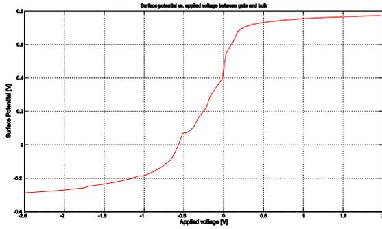
Figure 6. Plot of the surface potential versus the applied voltage. This function is technology dependant.
