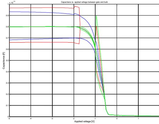
Figure 3. Fitting C-V curves by changing variables  $A_1$  (green),  $A_2$  (red) and  $A_3$  (blue) in accumulation and depletion regions.
