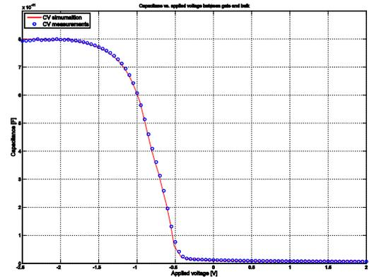
Figure 5. Plot of C-V simulation compared to experimental data after fitting. Highly accurate matching is achieved.
