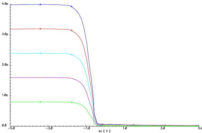
Figure 7. Plots of parametric  $C-V$  simulations for different values of dielectric thickness in extended bias range. The model behaves naturally as expected.
