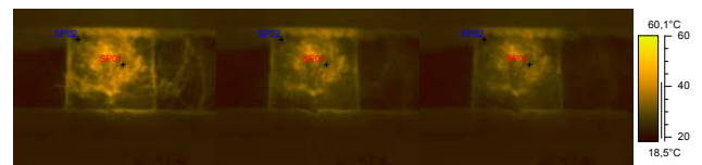
Fig. 3. Thermograms and dynamics of cooling for the steel object buried at 0,01 m depth in a sand test box
