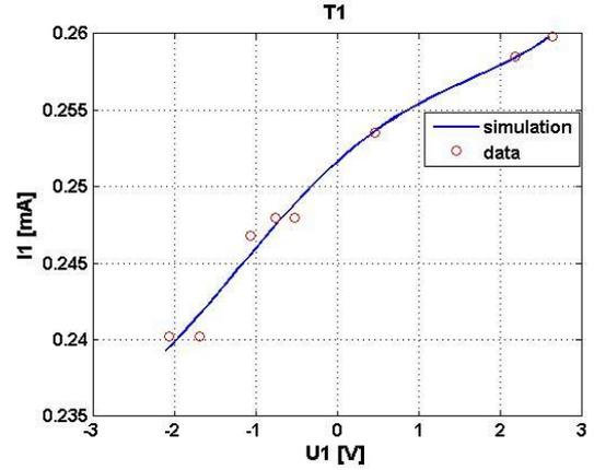
Figure 3.  $I$ - $V$  characteristic of block-element T1.
