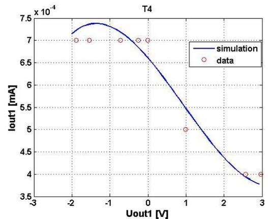
Figure 4.  $I$ - $V$  characteristic of block-element T4 (the first output of the microelectronic circuit).
