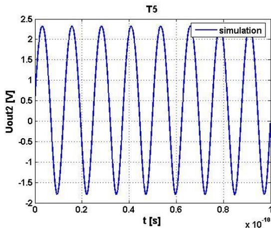
Figure 10. Output voltage at second output vs. time.
