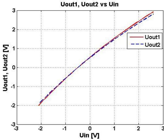
Figure 6. Output voltages at output 1 and output 2 vs. input voltage.
