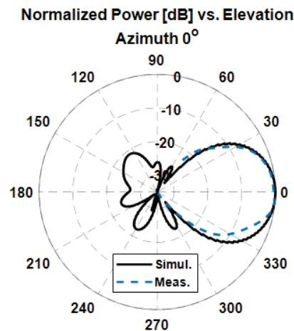
Fig. 9. Simulated and measured RP results in E-plane (elevation) for linear polarization
