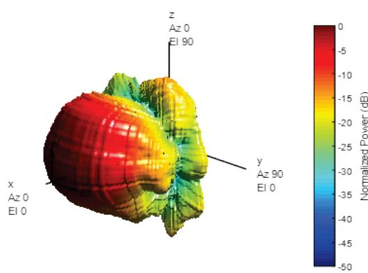
Fig. 14 Measured 3D RP for LHCP
