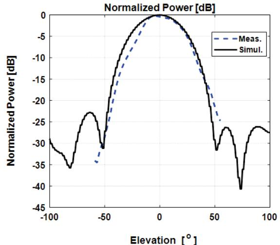
Fig. 10. Simulated and measured RP results in E-plane (elevation) for linear polarization
