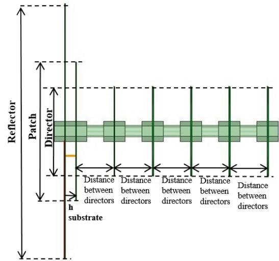
Fig. 1. Structure of the hybrid antenna with a suspended substrate
