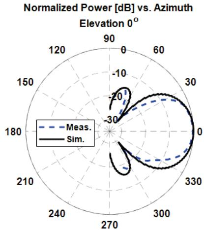
Fig. 7. Simulated and measured RP results in H-plane (azimuth) for linear polarization
