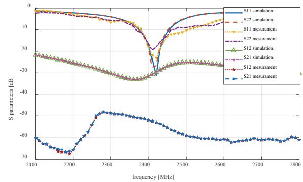
Fig. 5. S parameters of simulated and realized antenna
