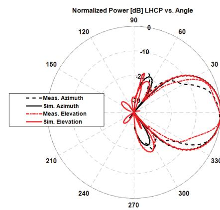
Fig. 11. Simulated and measured RP results in H and E planes for LHCP
