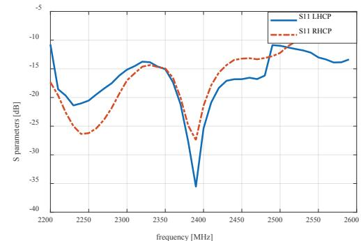
Fig. 6. Measured S11 parameters of the antenna with BLC feed network for CP
