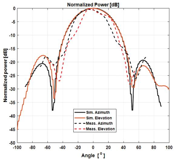
Fig. 12. Simulated and measured RP results in H and E planes for LHCP
