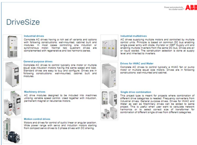
Fig. 3. Main screen of DriveSize Web – design toll of ABB
