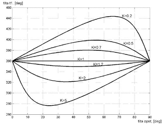
Fig.4 Electrical length of the resonator for the first spurious frequency
