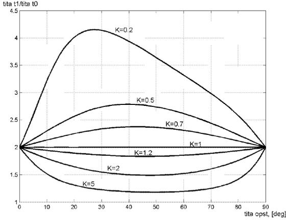
Fig.5. Ratio of the resonator lengths  $\theta_{i1}/\theta_{t0}$  as a function of the electrical length of the open stub.
