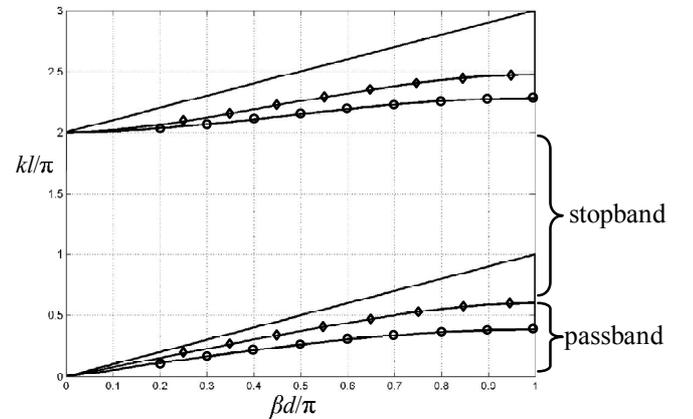
Fig.6 Dispersion curves for  $\theta_{opst} = \pi/6 rad$ ,  $Z_{opst} = 20\Omega$  (circles) and  $Z_{opst} = 40\Omega$  (diamonds), halfwave resonator-solid line
