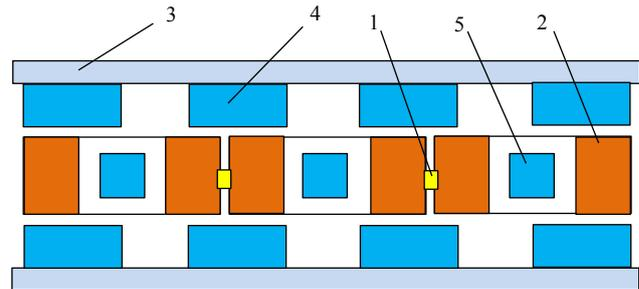
**Fig.1.** Generator with rotating magnets in its stator windings
